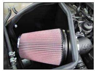
26. Install the K&N<sup>®</sup> air filter and secure with the provided hose clamp.
