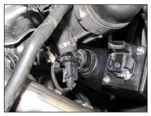
24. Connect the vent Quick disconnect fitting onto the fitting installed into the K&N<sup>®</sup> intake tube.
