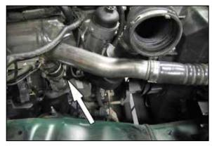
7. Loosen the hose clamp that secures the intake tube to the turbo inlet.
