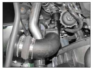
23. Install the K&N<sup>®</sup> intake tube into the coupler at the turbo and then into the coupler at the filter adapter, adjust the tube for best fit and then secure with the provided hose clamps.
