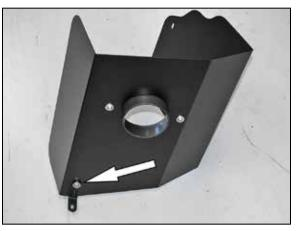
12. Install the mounting bracket (070015) onto the heat shield and secure with the provided hardware.
