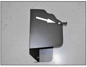
13. Install the provided bracket (07805) with spacer onto the heat shield and secure with the provided hardware.
