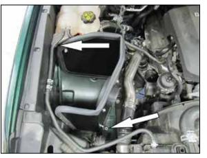
16. Install the heat shield and secure with the factory nut from the previous step and the hardware provided.
