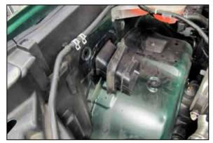
6. Remove the inlet duct from the inner fender.
