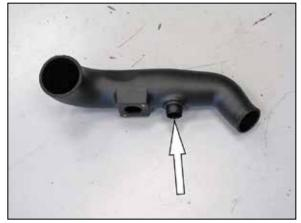
17. Install the provided grommet and quick disconnect fitting into the K&N<sup>®</sup> intake tube.
