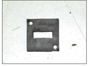
18. Install the provided gasket onto the K&N $^{\mbox{\tiny \$}}$  mass air sensor adapter.
