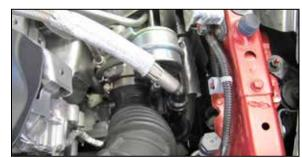
3. Disconnect the crank case vent hose.
