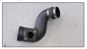
10. Install the provided hump coupler (084018) hose onto the  $K\&N^{\odot}$  intake tube and secure with the provided hose clamp.
