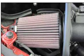
17. Install the air filter onto the  $K\&N^{\otimes}$  intake tube and secure with the provided hose clamp. Adjust the tube and heat shield for best fit and then secure them with the hose clamp and hardware.
