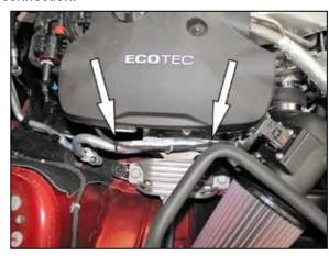
20. Using the provided tie wraps, secure the mass air sensor electrical cable to the A/C line as shown.
