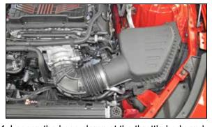
4. Loosen the hose clamp at the throttle body and then remove the complete stock intake system. NOTE: The air filter housing is snapped into three grommets.
