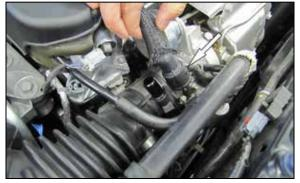
3. Snap the provided quick release tool onto the CCV tube, then push it up to unlock the CCV quick release connector and disconnect the CCV hose from the intake tube.
