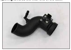
13. Install the provided guick disconnect fitting into the K&N® intake tube as shown.
