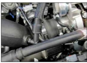
15. Connect the CCV hose to the quick disconnect fitting installed into the K&N® intake tube.
