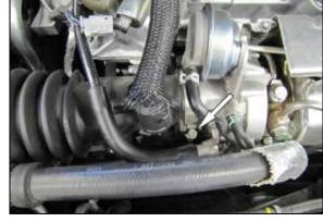
4. Loosen the hose clamp that secures the intake tube to the turbo inlet then disconnect the tube from the turbo. Lift the intake assembly up to dislodge it from the mounting grommets and then remove the complete intake system from the vehicle.
