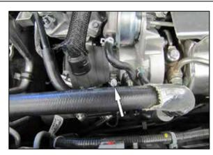
5. Install the provided coupler (5-1045) onto the turbo inlet and secure with the provided hose clamp.
