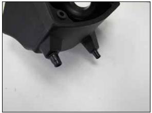
13. Remove the two factory mounting grommets from the factory air filter housing and install them onto the K&N® air filter housing.
