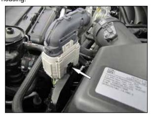
8. Using a small 90° pick or similar tool, release the locking tap that secures the wiring harness bulk connector to the air filter housing and then unhook the connector from the housing.
