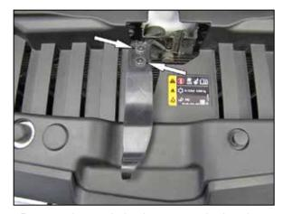
5. Remove the two bolts that secure the hood release arm to the hood latch and then remove the release arm.
