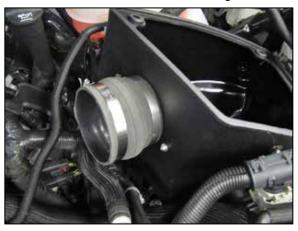
17. Install the provided hump coupler (08418) onto the filter adapter and secure with the provided hose clamp.
