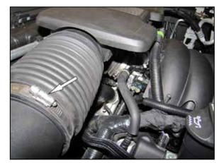
4. Loosen the hose clamps that secure the intake plenum assembly to the throttle body and air filter housing. Disconnect the plenum from the air filter housing and then rotate the plenum assembly counter clockwise to disengage the keyed mount and then remove the plenum from the throttle body. NOTE: Wiring harness anchored to plenum will need to be detached before removing from vehicle.
