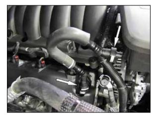
3. Depress the locking tabs and then disconnect the crank case vent line from the intake plenum and valve cover vent port.
