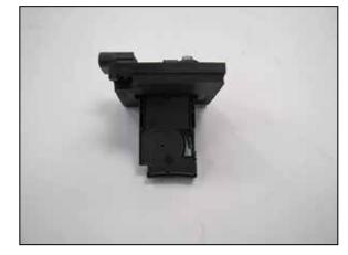
19. Install the provided gasket onto the provided mass air sensor adapter. Remove the mass air sensor from the factory air filter housing and then install it into the adapter and secure with the provide hardware.
