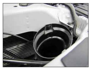
15. Push the factory fresh air intake duct into the K&N® air filter housing and then reinstall the plastic clip to secure it into position.
