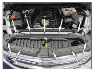
6. Release the ten plastic locking pins holding the upper radiator valence and then remove the valence from the vehicle.
