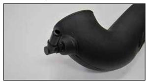
21. Install the 90° quick disconnect vent fitting into the K&N<sup>®</sup> intake tube as shown.
