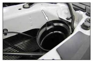
7. Remove the plastic clip securing the fresh air intake duct onto the core support, then pull the duct forward to disengage it from the factory air filter housing.
