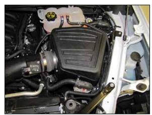
27. Install the K&N® air filter housing lid onto the air filter housing so the posts engage with the mounting grommets.
