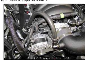
24. Install the crank case vent hose assembly onto the valve cover port and onto the 90° fitting on the intake tube.
