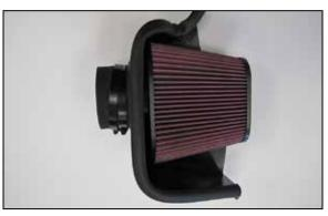
13. Install the K&N<sup>®</sup> air filter into the heat shield, install coupler hose (08761) onto the filter and secure with the provided hose clamp.
