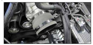
15. Install the provided coupler (08633) onto the throttle body and secure with the provided hose clamp.
