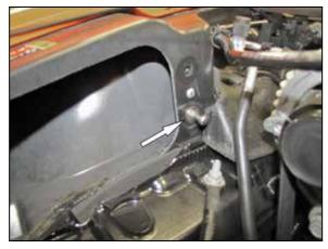
9. Remove the air filter housing mounting stud from the inner fender.
