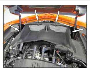
Loosen the four bolts that secure the air extractor duct to the radiator and then remove the
