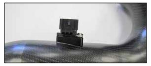
16. Remove the mass air sensor from the factory mass air sensor housing and install it into the K&N<sup>®</sup> intake tube using the provided hardware.
