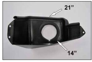
12. Install the edge trim onto the K&N $^{\mbox{\tiny \$}}$  heat shield as shown.
