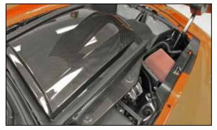
22. Reinstall the super charger cover and secure with the factory hardware.
