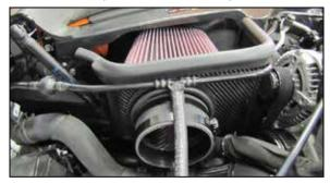
14. Install the heat shield/air filter assembly onto the rubber mounted studs and secure with the provided hardware.
