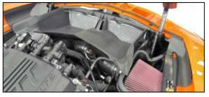
21. Reinstall the air extractor duct and secure with the factory hardware.
