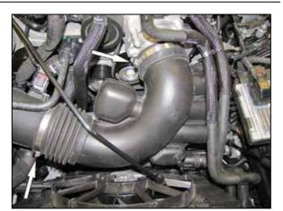
5. Loosen the two hose clamps that secure the factory intake tube and then remove the intake tube
