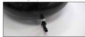
17. Install the provided crank case quick connect fitting into the K&N<sup>®</sup> intake tube as shown. **NOTE: Plastic NPT fittings are easy to cross thread. Install the vent fitting "hand" tight, then turn it two complete turns with a wrench.**
