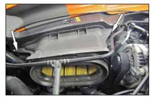
8. Remove the two bolts that secure the air filter housing to the inner fender and then remove the housing and air filter from the vehicle. **NOTE: K&N Engineering, Inc., recommends that customers do not discard factory air intake.**
