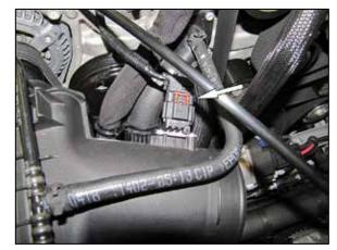
6. Pull the red locking tab back and then disconnect the mass air sensor electrical connection.
