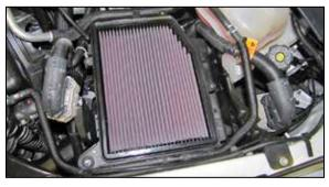
5. Remove the upper air filter housing and replace the factory air filter with the provided K&N® air filter and then reinstall the upper housing and secure with the factory hardware.
