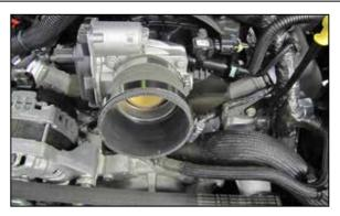
7. Install the provided straight coupler (084055) onto the throttle body and secure with the provided hose clamp.
