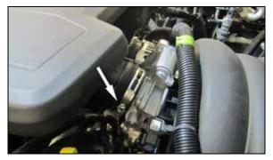
4. Loosen the hose clamp that secures the intake plenum to the throttle body. Rotate the plenum counter clockwise to unlatch it from the mounting bracket and then remove the plenum from the vehicle
