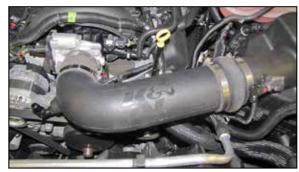
9. Install the K&N® intake tube into the coupler at the air filter housing and then into coupler on the throttle body, adjust the tube for best fit and then secure with the provided hose clamps.
