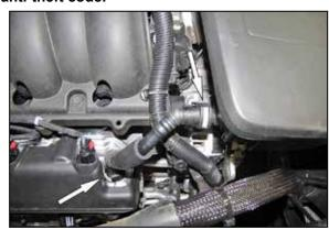
2. Depress the locking tabs and disconnect the crank case vent line from the intake plenum and valve cover.
