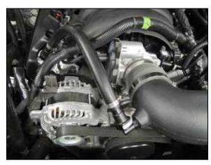
11. Connect the crankcase vent hose assembly to the fitting in the K&N® intake tube and to the valve cover port.
