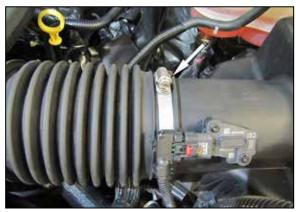
3. Loosen the hose clamp that secures the intake tube to the air filter housing.
