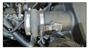
6. Install the provided hump coupler (08418) onto the air filter housing and secure with the provided hose clamp.
