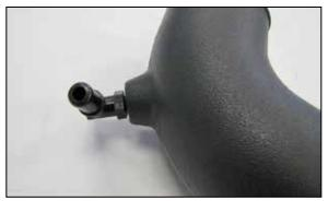
8. Install the provided 90° vent fitting into the K&N° intake tube as shown.
