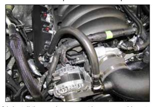
24. Install the crank case vent hose assembly onto the valve cover port and onto the 90° fitting on the intake tube.
