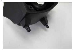
13. Remove the two factory mounting grommets from the factory air filter housing and install them onto the  $K\&N^{\otimes}$  air filter housing.
