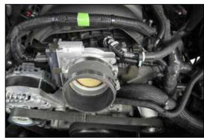
18. install coupler (084055) onto the throttle body and secure with the provided hose clamp.
