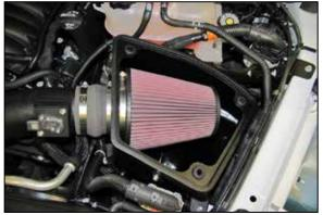
25. Install the K&N® air filter onto the filter adapter and secure with the provided hose clamp.
