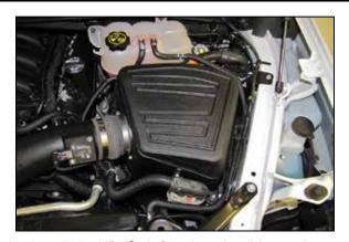
27. Install the K&N® air filter housing lid onto the air filter housing so the posts engage with the mounting grommets.
