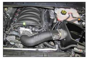
23. Install the K&N® intake tube into the coupler at the air filter housing and then into the coupler on the throttle body, adjust the tube for best fit and then secure with the provided hose clamps.
