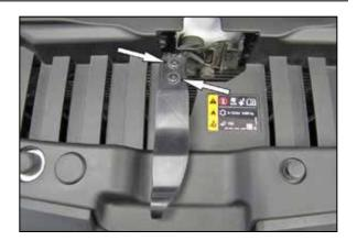
5. Remove the two bolts that secure the hood release arm to the hood latch and then remove the release arm.
