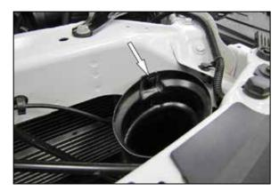
7. Remove the plastic clip securing the fresh air intake duct onto the core support, then pull the duct forward to disengage it from the factory air filter housing.
