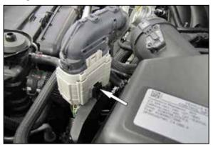
8. Using a small 90° pick or similar tool, release the locking tap that secures the wiring harness bulk connector to the air filter housing and then unhook the connector from the housing.
