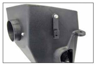
12. Install the provided wiring harness bracket onto the K&N® air filter housing and secure with the provided hardware.
