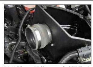
17. Install the provided hump coupler (08418) onto the filter adapter and secure with the provided hose clamp.
