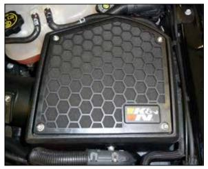
27. Install the prefilter and cage onto the air filter housing and secure with the provided hardware and then install the K&N badge into the cage as shown.
