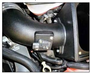
23. Install the intake tube into the coupler and align with the filter housing, then slide the gasket between the tube and housing, insert the filter adapter through the housing and gasket into the intake tube. Align the mounting holes and then secure with the provided hardware.
