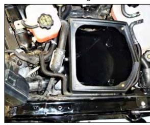
16. Install the K&N air filter housing into the vehicle so the mounting grommets insert into the factory mounting holes and then secure with the factory mounting nut.
