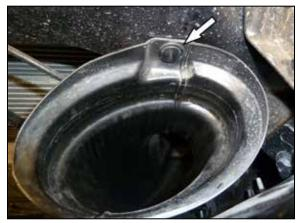
4. Remove the retaining clip shown that secures the fresh air duct and then disconnect the duct from the air filter housing.
