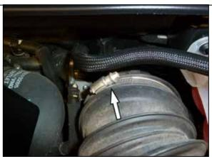
5. Loosen the hose clamp that secures the intake hose to the turbo inlet and disconnect the hose from the inlet.
