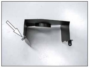
8. Install the mounting bracket (070066A) onto the heat shield using the provided hardware.
