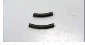
21. Cut the provided crank case vent hose into two sections, one section will be 5" long and the other will be 6-1/2" long.
