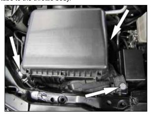
6. Remove the three bolts that secure the air filter housing to the inner fender and then remove the complete intake system from the vehicle.
