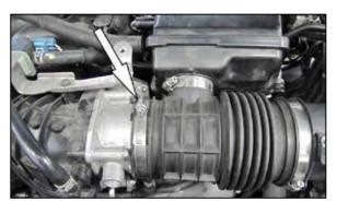
5. Loosen the hose clamp that secures the intake tube to the throttle body.
