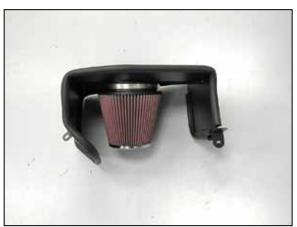
11. Install the K&N® air filter onto the filter adapter and secure with the provided hose clamp.
