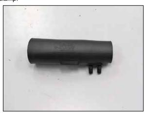
15. Install the two provided NPT vent fittings into the  $K\&N^{\odot}$  intake tube as shown.
