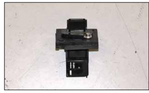
18. Install the mass air sensor into the K&N® adapter and secure with the provided hardware.
