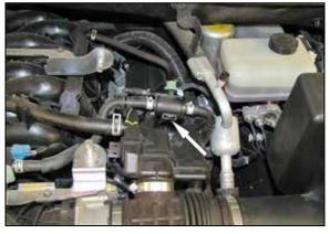
4. Unclip the EVAP line and test port from the factory intake tube.
