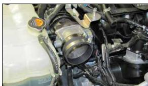
17. Install the provided coupler hose (08698) onto the throttle body and secure with the provided hose clamp.
