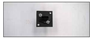
16. Remove the mass air sensor from the factory housing and install it into the K&N® mass air sensor adapter and secure with the provided hardware.
