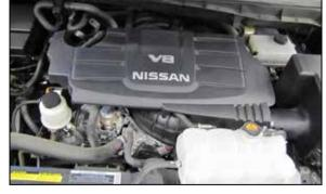
3. Lift up the engine cover and remove it from the vehicle.
