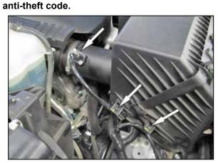
2. Disconnect the mass air sensor electrical connection and then unclip the harness from the air filter housing.
