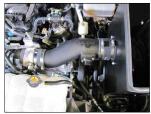
19. Install the provided coupler (08698) onto the intake tube (Do not tighten). Install the intake tube into the coupler at the throttle body and align with the filter adapter. Secure the coupler hose and intake tube with the provided hose clamps.
