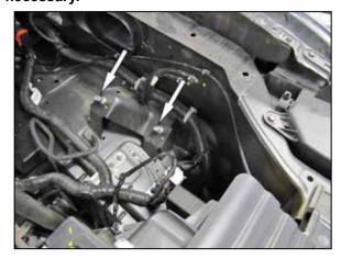
11. Remove the two-factory air filter housing mounting studs from the inner fender.
