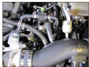
21. Install the vent fittings into the factory vent hoses and then onto the fittings installed into the K&N® intake tube.
