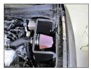
23. Install the K&N® air filter and secure with the provided hose clamp.
