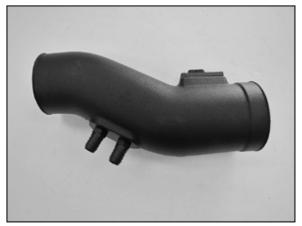
14. Install the two provided vent fittings into the K&N® intake tube as shown.
