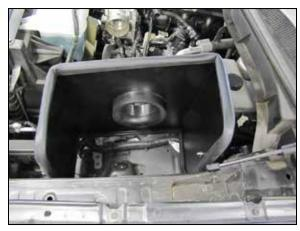
13. Install the heat shield onto the inner fender and secure with the provided hardware.
