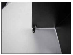
8. Install the provided mounting bracket (070712A) onto the heat shield using the provided hardware.
