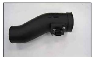
18. Install the mass air sensor assembly into the K&N® intake tube and secure with the provided hardware.
