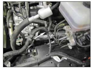
12. On 4 wheel drive models, secure the front differential vent line to the EVAP vent line.
