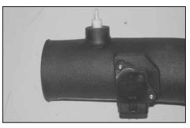
24. Install the vent fitting into the K&N $^{\circ}$  intake tube as shown.
