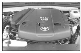
2. Loosen the two nuts that secure the engine cover, then remove the engine cover.
