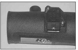
23. Secure the mass air sensor to the K&N^{\otimes} intake tube using the provided screws and spacers as
