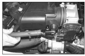
8. Remove the crank case vent hose from the air box as shown.
