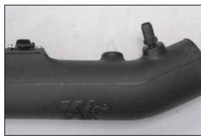
26. Install the 5/8 vent fitting into the K&N® intake tube as shown.
