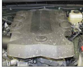
34. Reinstall the engine cover onto the engine.
