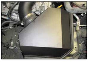
33. Install the heat shield cover onto the heat shield and secure with the provided hardware.
