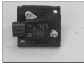
24. Install the mass air sensor into the K&N® mass air sensor adapter and secure with the provided hardware.
