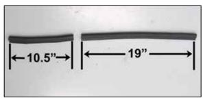
17. Cut the provided edge trim into two lengths as shown. One section is to be 10.5" long and one section is to be 19" long.
