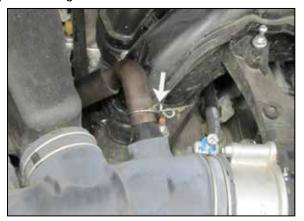
5. Disconnect the crank case vent hose from the stock intake tube.
