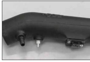
27. Install the 3/16 vent fitting into the K&N® intake tube as shown.
