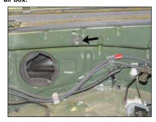
13. Install the 6mm rubber mounted stud into the inner fender location shown.
