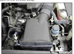
8. Release the four clips which secure the upper air box to the lower air box and then remove the intake tube and upper air box from the vehicle.
