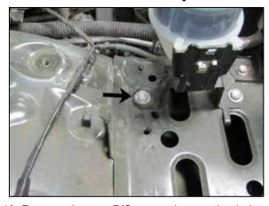
10. Remove the rear P/S reservoir mounting bolt shown.
