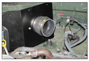
20. Install the provided silicone hump hose (084057) onto the filter adapter and secure with the provided hose clamp.
