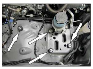
12. Install the four rubber mounted studs into the factory air box and P/S reservoir as shown.
