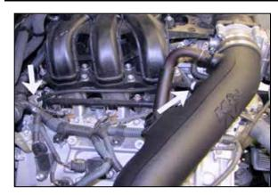
30. Connect the provided fuel pressure vent line to the fuel pressure regulator and then connect the open end to the 3/16 vent fitting in the K&N® intake tube.
