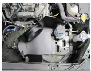
19. Set the heat shield onto the rubber mounted studs and the secure with the provided hardware. NOTE: On models that had a horn attached in this location, be sure to reattach the horn between the heat shield bracket and rubber mounted stud.
