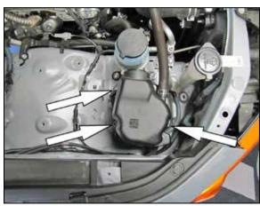
11. On models with the Air injection pump located in front of the air box next to the Power steering reservoir, remove the three bolts securing the pump to the inner fender.
