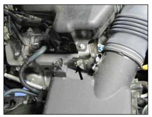
6. Remove the bolt which secures the tube mounting bracket to the engine valve cover.
