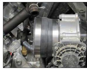
21. Install the provided silicone step hose (084091) onto the throttle body and secure with the provided hose clamp.
