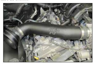
28. Install the K&N® intake tube into hump hose at the filter adapter and then into the silicone hose at the throttle body, align the tube for proper fit and then tighten the hose clamps.
