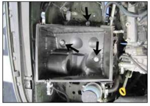
9. Loosen and remove the three bolts securing the lower air box and then remove the lower air box from the vehicle.
