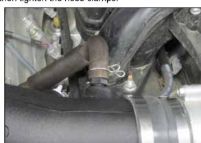
29. Connect the crank case vent line to the 5/8 vent fitting and secure with the factory spring clamp.
