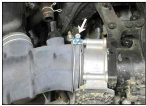
7. Loosen the hose clamp which secures the intake tube to the throttle body.
