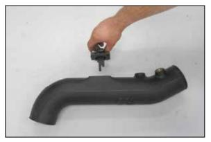
25. Install the mass air sensor assembly into the K&N® intake tube and secure with the provided
