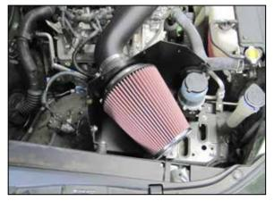
31. Install the K&N® air filter onto the filter adapter and secure with the provided hose clamp.
