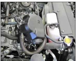
11a. Lift up the air injection pump, disconnect the electrical connection and then set the air injection pump over to side.
