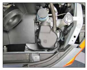
19a. Install the air injection pump onto the heat shield and forward rubber mounted stud and then secure with the provided hardware. Reconnect the air injection pump electrical connection.
