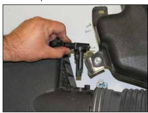
23. Remove the screws which secure the mass air sensor to the factory air box and then remove the mass air sensor from the air box.
