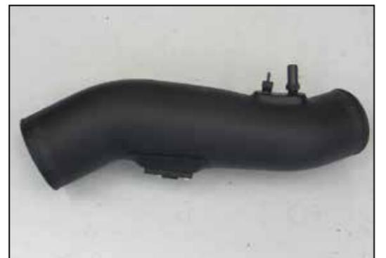
24. Install the provided NPT vent fittings into the K&N® intake tube as shown.
