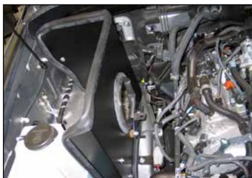
19. Set the heat shield into position on the inner fender and then secure with the factory bolt removed in step #18 with the provided hardware.
