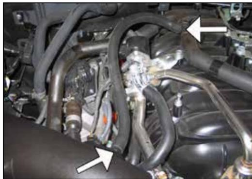
31. Install the provided crankcase vent line onto the NPT fitting installed into the K&N® intake tube and connect the open end onto the factory Tee.
