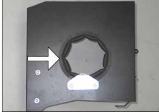
16. Install the provided shorter edge trim into the hole of the heat shield as shown.
