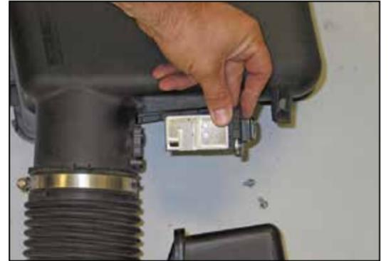
21. Remove the mass air sensor from the factory airbox.
