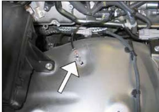
18. Remove the bolt that secures the ground strap to the inner fender.
