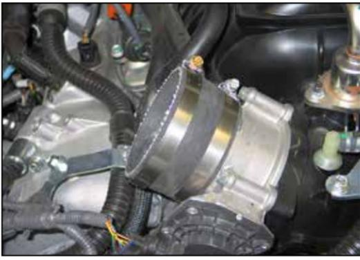
25. Install the provided silicone (08630) hose onto throttle body and secure with the provided hose clamp.
