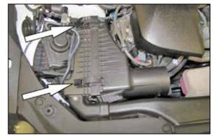
6. Install the K&N® air filter and then resecure the clean side housing.
