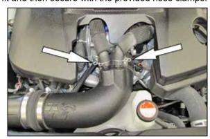
11. Install the crank case breather hoses and then secure with the factory spring clamps.
