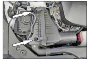
4. Release the two clips retaining the clean side of the filter housing.
