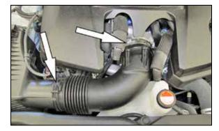
3. Loosen the hose clamps that secure the intake tube to the throttle body and air filter housing and then remove the intake tube from the vehicle. NOTE: K&N Engineering, Inc., recommends that customers do not discard factory air intake.
