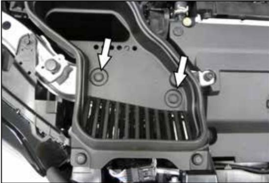
2. Push down the center of the two retaining pins to unlock them, then lift the complete fresh air duct assembly and remove it from the vehicle.
