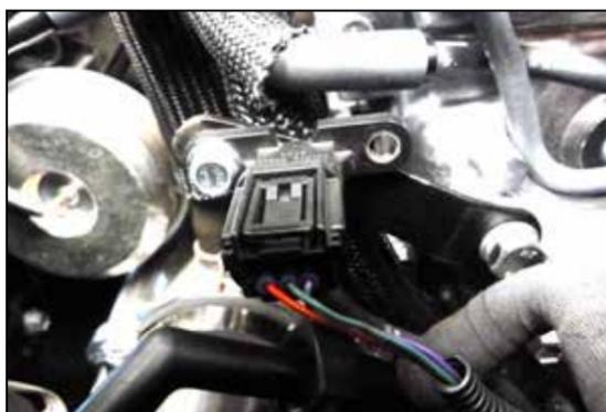
28. Using the provided bracket and hardware, mount the vacuum sensor to the engine as shown and then connect the vacuum line from the tee fitting connected to the ejector fitting.
