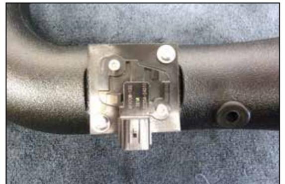
17. Install the maf assembly into the K&N intake tube, be sure to install the assembly in the correct orientation with the opening towards the air filter end of the tube.
