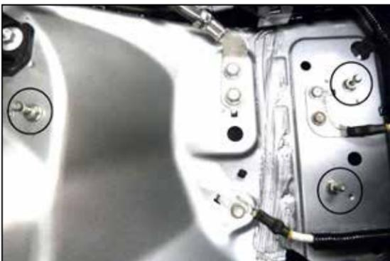
6. Remove the three air-filter housing mounting studs shown.
