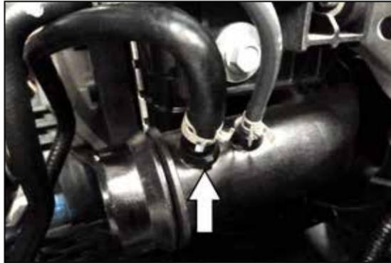
8. Release the spring clamp that secures the vent line shown to the charge tube manifold and then disconnect the hose from the manifold.
