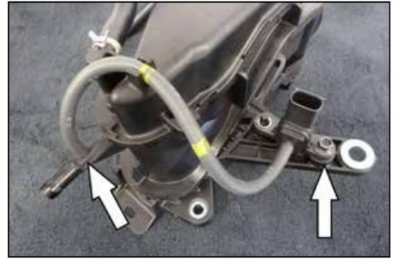
12. Disconnect the vacuum line shown, remove the sensor mounting bolt and then remove the sensor.
