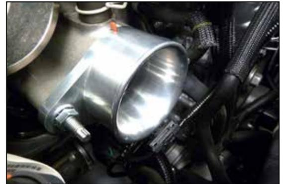
14. Install the K&N turbo inlet onto the turbo and secure with the factory mounting nuts.
