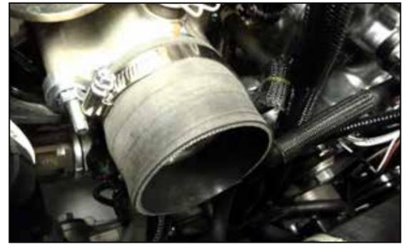
15. Install the provided coupler onto the turbo inlet and secure with the provided hose clamp.
