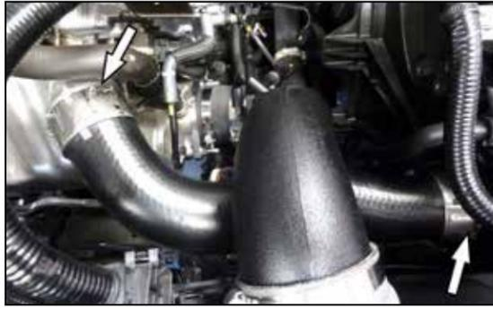
24. Reinstall the charge tube and secure with factory retaining clips.
