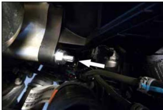
10. Remove the two manifold mounting nuts and then slide the housing off the turbo inlet.
