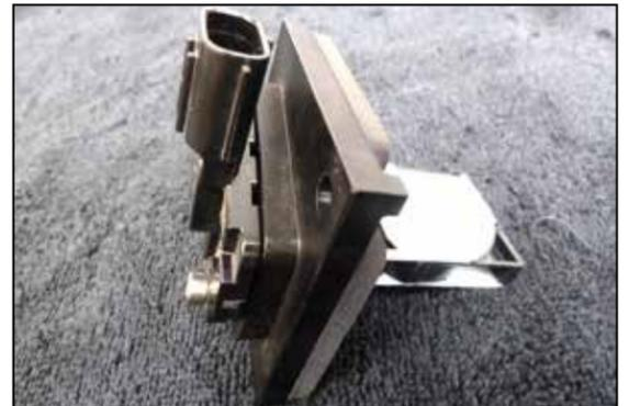
16. Install the gasket onto the K&N maf adapter. Remove the maf sensor from the factory housing and install it into the K&N adapter and secure with the provided hardware.
