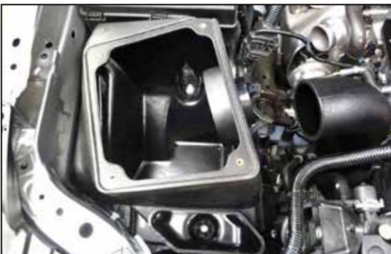
22. Install the K&N air filter housing assembly into the vehicle and secure with the provided hardware.
