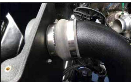
23. Install the provided hump coupler onto the intake tube and filter adapter, align for best fit and then secure with the provided hose clamps.
