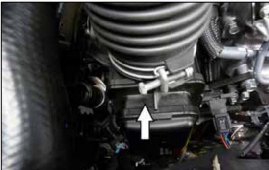
4. Loosen the hose clamp that secures the factory intake tube to the turbo inlet.
