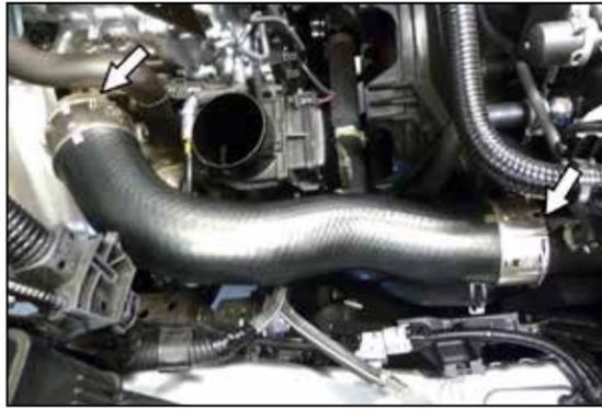
7. Release the spring clips that secure the charge tube quick connect fittings and then remove the charge tube assembly from the vehicle.
