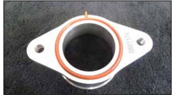
13. Remove the sealing O-ring from the factory turbo manifold and install it into the K&N turbo inlet flange.
