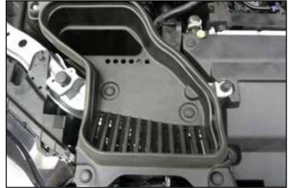
31. Reinstall the factory fresh air duct and secure with the factory pins.
