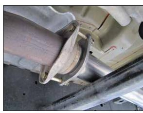
5. Install the K&N® mid-pipe and secure with the provided hardware. Do not tighten the flange mounting bolts at this time.
