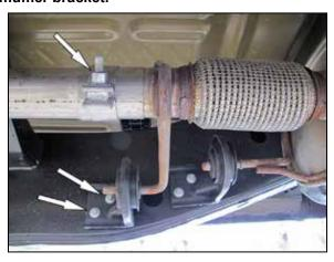
4. On vehicles equipped with a 2.7L / 3.5L Ecoboost V6, remove the two bolts that secure the front exhaust mount to the frame, this mount will not be used with the K&N® exhaust system. Slide the entire exhaust system towards the rear of the vehicle to unhook the remaining hangers and then route the exhaust forward over the axle and out from the vehicle. NOTE: The stock muffler can be disconnected from the stock mid pipe at the connection shown if desired to ease system
