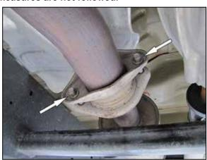
2. Remove the two bolts that secure the factory connection between the tail pipe and head pipe. NOTE: K&N Engineering, Inc., recommends that customers do not discard factory exhaust.
