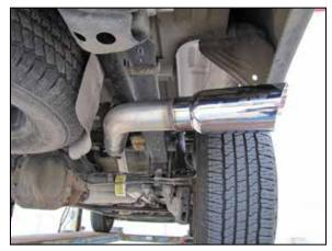
8. Check alignment and reposition as necessary. Once final position is satisfactory, tighten all hardware and band clamps from front to rear of
