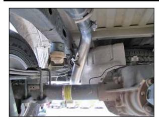
7. Install the tail pipe onto the muffler and attach the tail pipe hangers.
