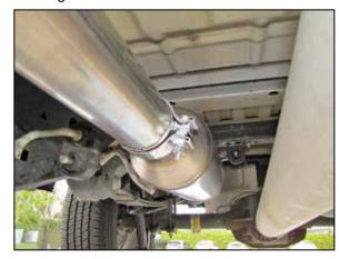
6. Install the K&N® muffler onto the mid-pipe and install the factory muffler hangers onto the muffler. NOTE: Do not tighten the muffler connection at this time.
