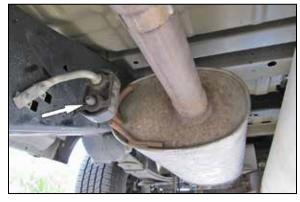
3. On vehicles equipped with a 5.0L V8, unhook the exhaust hanger from the muffler bracket. Slide the entire exhaust system towards the rear of the vehicle to unhook the remaining hangers and then route the exhaust forward over the axle and out from the vehicle.
