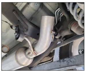
10. Slide mid pipe muffler assembly into position on the vehicle by first using the hangers on the muffler end. Once inserted, then slide assembly rearward allowing the mid pipe to seat against head pipe.
