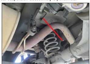
3. Cut rear tailpipe 2" from rear hanger just above the axle.
