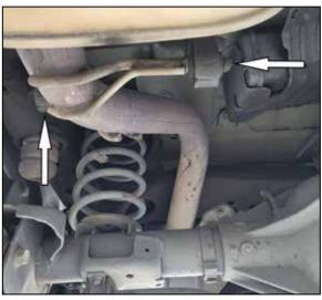
6. Remove muffler assembly from remaining hangers starting with the front hanger.
