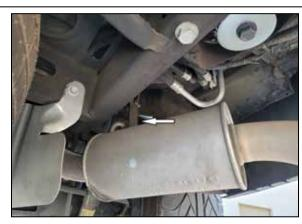
4. Remove rear tail pipe section by sliding tail pipe off rear hanger (leave rubber hanger on vehicle).
