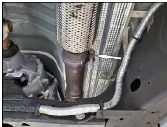
4. Once rear tail pipe has been removed loosen front conical clamp connecting tail pipe to head pipe.
