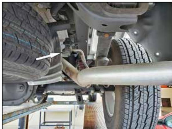
3. Remove rear tail pipe section by sliding tail pipe off rear hanger (leave rubber hanger on vehicle).
