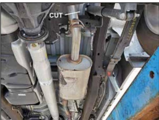
2. Unless a vehicle lift is available cutting the stock exhaust will be mandatory to remove. Cut rear tailpipe 2" from rear hanger just above the axle where shown.
