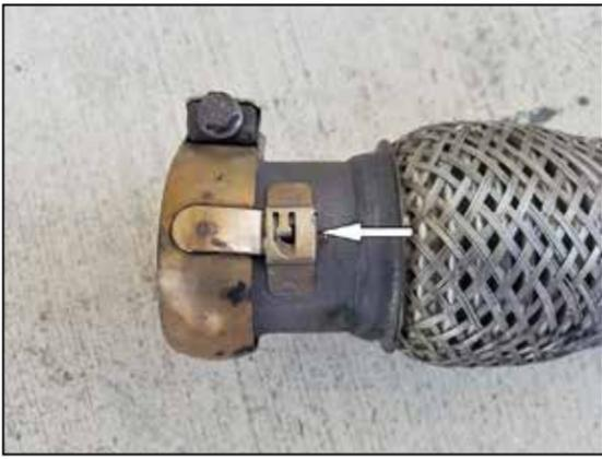
7. Once stock system is removed, remove the conical clamp by prying retaining tang upwards.
