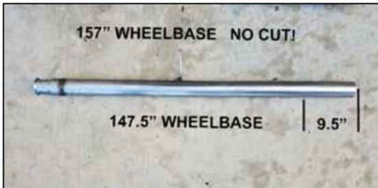
8. For vehicles with 147.5" wheelbase 9.5" must be cut off the end opposite to the conical end connecting to the head pipe (As shown). For vehicles with 157" wheelbase it does not need to be cut.
