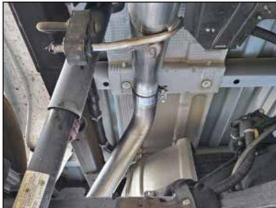
12. Slide band clamp on to the front of the tail pipe section. Then slide tail pipe section into muffler section.
