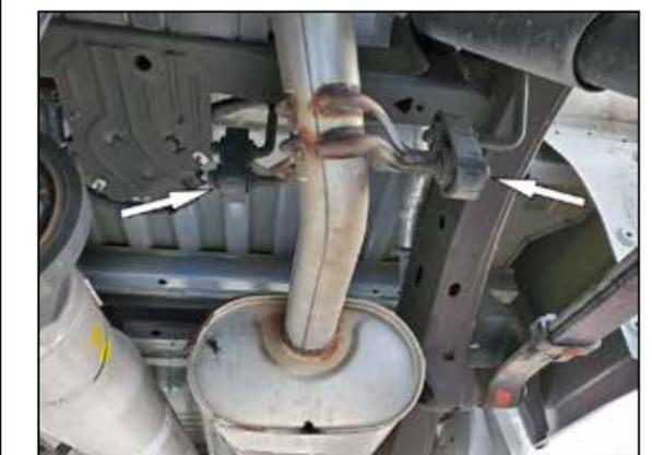
5. Remove muffler assembly from remaining hangers.
