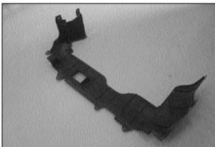
7. From underneath the vehicle, carefully remove the splash guard.
