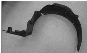
8. Unscrew and remove the right inner fender well.
