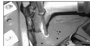
17. Fit the two bend short intake tube into the hump hose. Align its welded on bracket with the threaded air box mounting hole in the chassis leg and secure it with the M6 bolt and wave washer supplied as shown.
