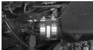
12. Fit the silicone hose to the throttle body housing using the #40 hose clamp supplied.
