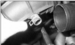
3. Unclip and remove the breather hose from the intake hose as shown.
