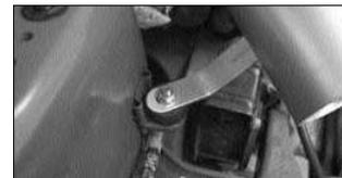
14. Align the welded on bracket to the vibration mount for best overall fit and clearance and secure using the M6 nylock nut and wave washer supplied.
