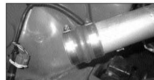
16. Fit the silicone hump hose to the intake tube using the #40 hose clamp supplied. Make sure the tube is inserted about 1 7/2.5 cm into the hose.
