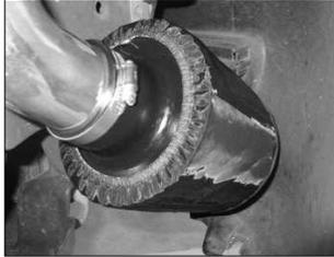
20. Fit the filter to the intake tube and secure the hose clamp supplied.
