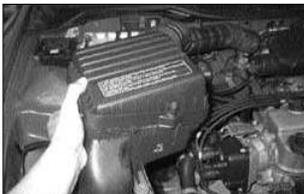
5. Unbolt the three bolts and remove the complete air box assembly from the vehicle.
