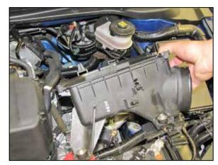
7. Remove the two bolts securing the lower air filter housing to the vehicle. Disconnect the transmission breather hose from the lower air filter housing. Lift up the housing to dislodge it from the rear mounting grommet and then remove the housing from the vehicle.
