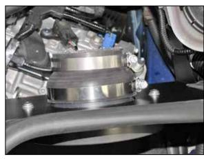
17. Install the provided step coupler (084093) onto the filter adapter and secure with the provided hose clamp.
