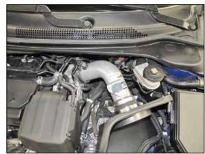
20. Install the K&N® intake tube into the coupling hoses and adjust the tube for best fit then secure with the provided hose clamps.
