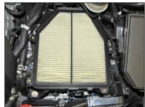
6. Remove the factory air filter.
