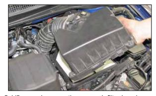
5. Lift up and remove the upper air filter housing and remove it from the vehicle.
