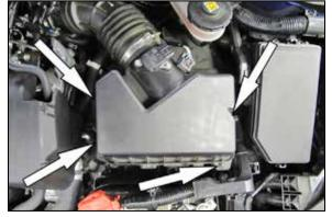
4. Loosen the four screws securing the upper air filter housing and disconnect the wiring harness from the housing.
