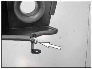
14. Install the vent hose clip into the heat shield as shown.
