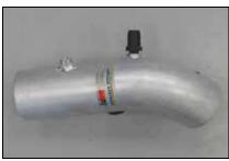
16. Install the provided NPT fitting into the K&N® intake tube as shown.
