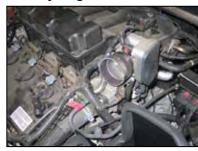
20. Install the provided silicone hose (084036) onto the throttle body and secure with the provided hose clamp.
