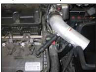
22. Install the provided crankcase vent hose onto the fitting on the valve cover. Then connect the open end to the NPT fitting installed into the K&N<sup>®</sup> intake tube.
