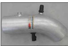
19. Install the inlet air temperature sensor into the grommet installed into the K&N® intake tube.
