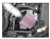
24. Install the K&N® air filter onto the intake tube and secure with the provided hose clamp.
