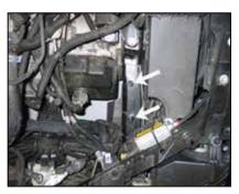
8. Remove the two airbox mounting studs from the frame rail.
