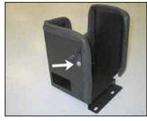
11. Install the heat shield mounting bracket (26517) onto the heat shield as shown using the provided hardware.
