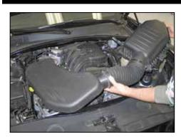
7. Remove the complete stock intake system from the vehicle.
