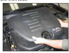
2. Lift up and remove the engine cover and remove it from the engine.
