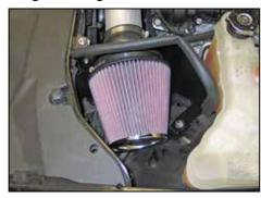
25. Install the K&N® air filter and secure with the provided hose clamp.
