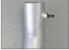
17. Install the inlet air temperature sensor into the K&N® intake tube as shown, turning the sensor clockwise to lock.
