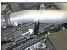
22. Install the tube bracket onto the mounting stud and then secure to the K&N® intake tube with the provided hardware. Tighten the hose clamps at this time
