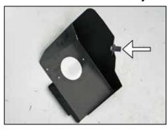
8. Install the inserted nut onto the heat shield using the provided hardware as shown.
