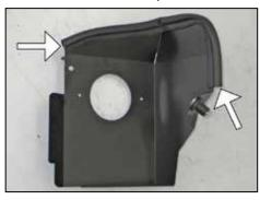
10. Install the provided longer edge trim onto the top of the heat shield as shown.
