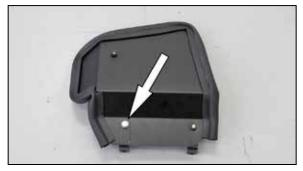
13. Flip the heat shield over and install the remaining bracket #070812 and secure with the provided hardware.
