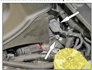
6. Disconnect the inlet air temperature sensor electrical connection and then loosen the hose clamp securing the intake plenum to the throttle body.
