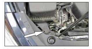
4. Remove the bolt securing the air filter housing onto the core support and unhook the coolant line from the air box.
