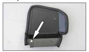
12. Install one of the provided brackets #070812A onto the heat shield as shown using the provided hardware.
