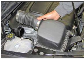
5. Lift up and remove the air filter housing assembly from the vehicle.
