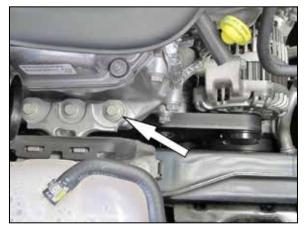
16. Remove the front engine mounting bolt shown.
