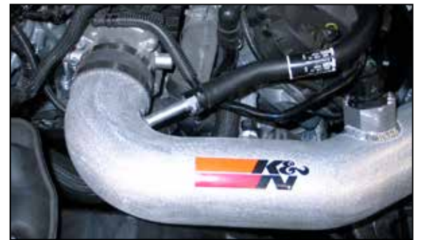
24. Connect the crank case vent hose to the fitting on the K&N® intake tube. NOTE: On vehicles equipped with an EVAP vent line: Connect the EVAP line to the fitting installed in the K&N® intake tube.
