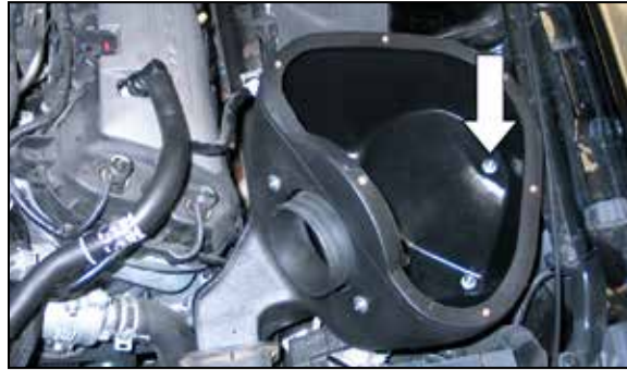
17. Set the K&N® air box into the vehicle so that the mounting studs slide into the mounting holes, then secure with the provided hardware.
