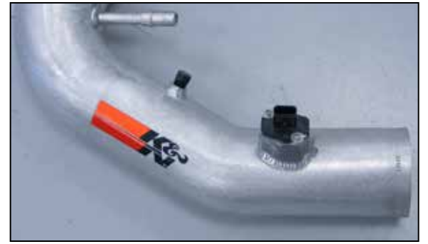
22. Install the mass air sensor into the K&N® intake tube and secure with the provided hardware.
