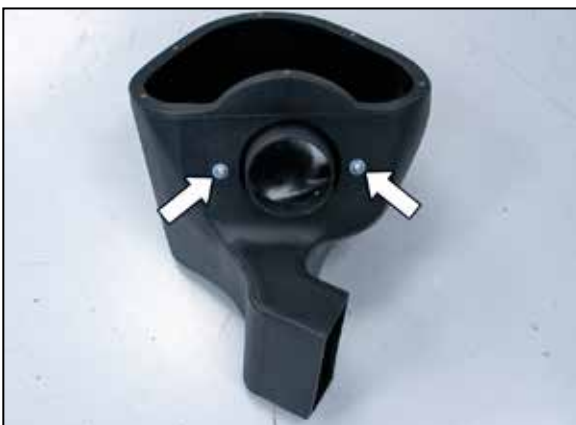
14. Install the filter adapter into the air box and secure with the provided hardware.
