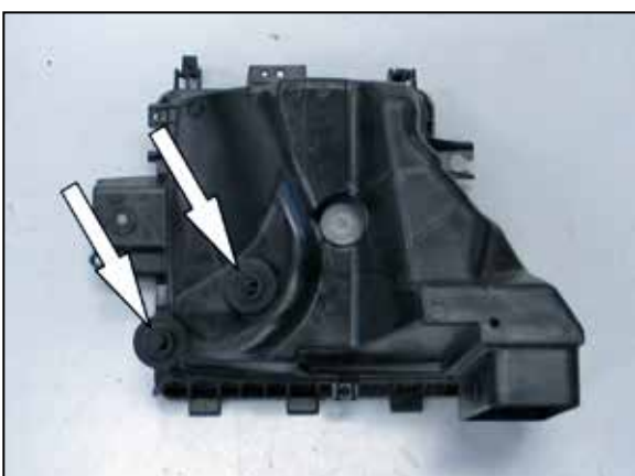
15. Remove the two air box mounting grommets from the factory air box.
