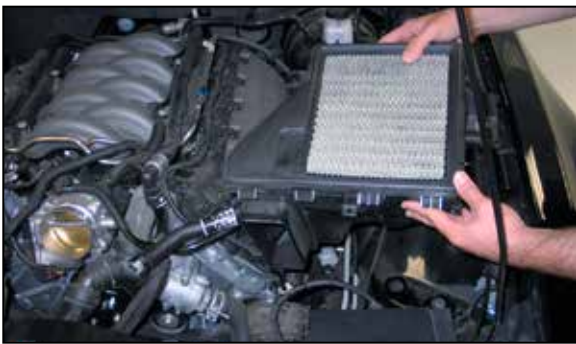
12. Remove the lower air box from the vehicle. NOTE: K&N Engineering, Inc., recommends that customers do not discard factory air intake.
