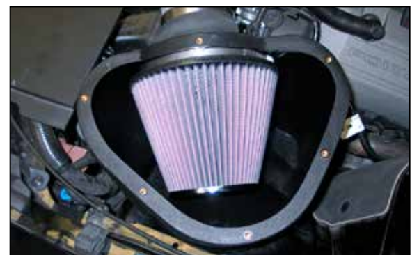
26. Attach the K&N® air filter onto the filter adapter and secure with the provided hose clamp.
