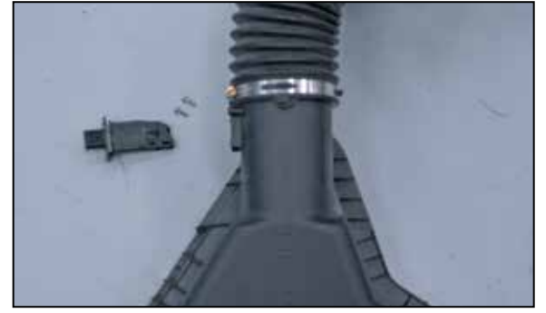
21. Remove the two bolts securing the mass air sensor into the factory intake tube and then remove the mass air sensor from the intake tube.
