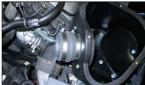
18. Install the provided silicone hose (08699) onto the filter adapter and secure with the provided hose clamp.
