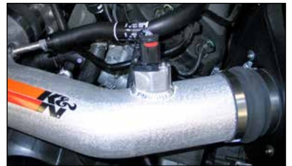
25. Reconnect the mass air sensor electrical connection.
