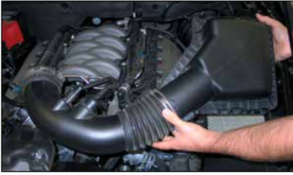
10. Remove the upper air box and intake tube from the vehicle.
