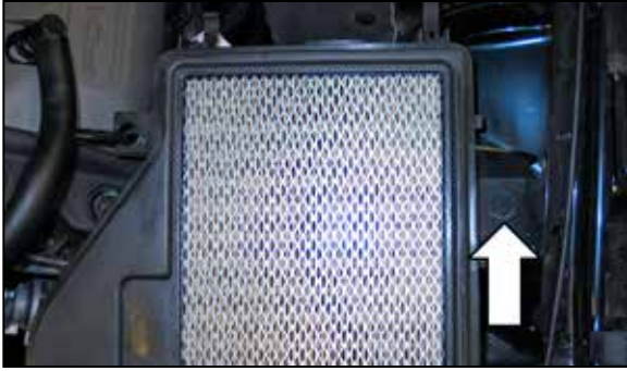
11. Remove the bolt that secures the lower air box to the inner fender.
