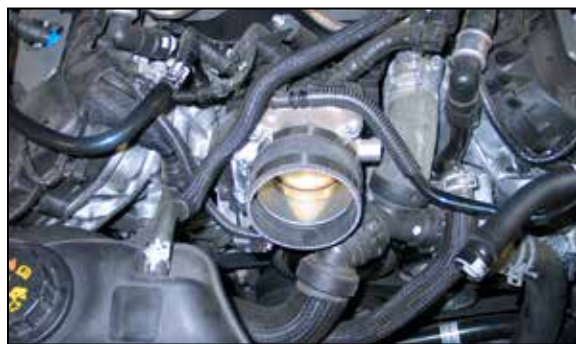
19. Install the provided silicone hose (08698) onto the throttle body and secure with the provided hose clamp.
