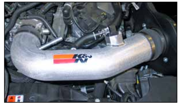
23. Install the K&N® intake tube into the silicone hose at the air box and then into the silicone hose at the throttle body; secure with the provided hose clamps.
