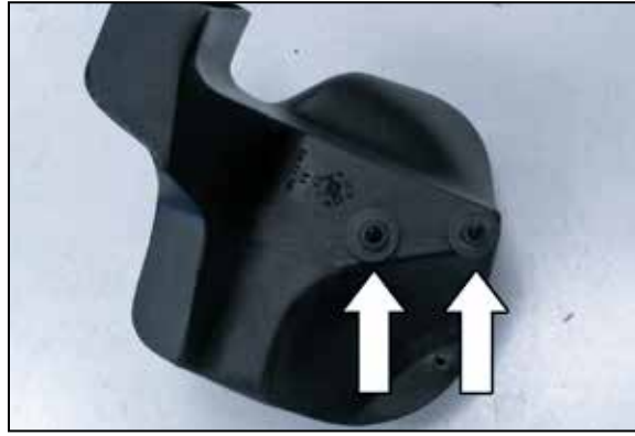
16. Install the air box mounting grommets onto the two mounting studs installed onto the K&N® air box.
