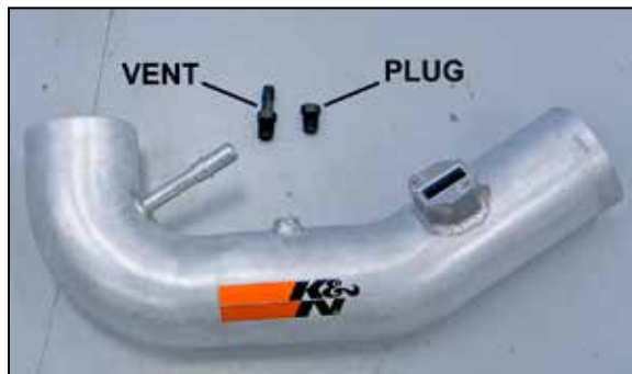
20. On vehicles that have an EVAP vent line attached to the intake tube, install the 3/8" vent fitting into the K&N® intake tube. On vehicles that do not have the EVAP vent line attached to the intake tube, install the npt plug into the intake tube. NOTE: Plastic NPT fittings are easy to cross thread. Install the vent fitting "hand" tight, then turn it two complete turns with a wrench.
