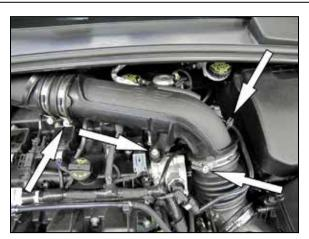
3. Remove the bolt securing the factory intake tube to the engine shown. Next loosen the hose clamps and unhook the vent line from the intake tube and
