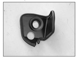
9. Install the provided edge trim onto the heat shield.
