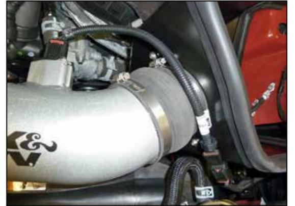
17. Reconnect the mass air sensor electrical connection using the provided extension harness.
