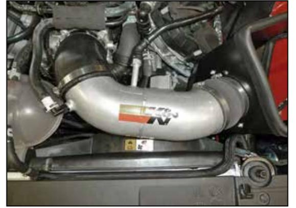
16. Install the intake tube into the coupler at the throttle body and onto the coupler at the filter adapter, adjust the tube for best fit and then secure the tube to the coupling hoses with the provided hose clamp. Connect the EVAP and crank case vent lines to the fittings installed into the K&N® intake tube.
