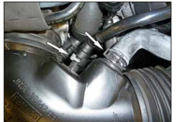
5. Disconnect the vent lines and sound tube attached to the intake tube. Loosen the hose clamps that secure the intake tube to the air filter housing and throttle body and then remove the intake tube from the vehicle.
