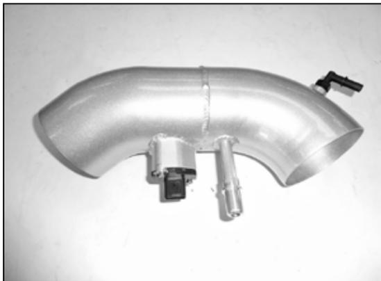
15. Install the provided 90° fitting into the K&N® intake tube. Remove the mass air sensor from the factory housing and install it into the K&N® intake tube using the provided hardware.
