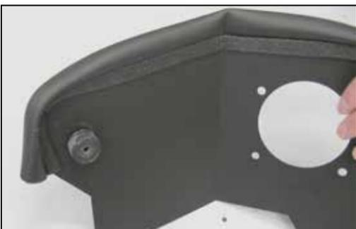
13. Install the remaining rubber mounted stud onto the heat shield as shown and secure with the provided hardware.
