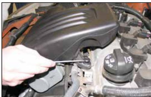
4. Using a small screw driver, release the plenum locking clip by prying the center of the plenum locking clip.
