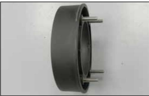
10. Install the four m6 studs into the threaded inserts in the filter adapter as shown.
