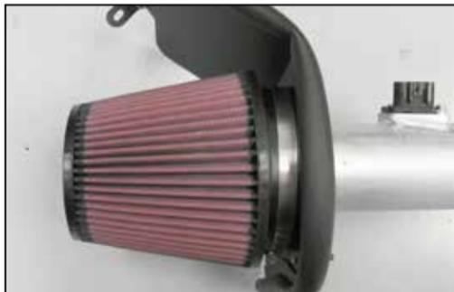
19. Install the K&N® filter onto the filter adapter and secure with the provided hose clamp.
