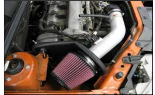
21. Install the K&N® intake tube into the silicone hose at the throttle body and align the "L" bracket with the inner airbox mounting stud as shown.
