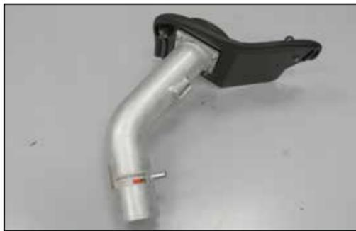
16. Install the K&N® intake tube to the filter adapter studs with the remaining gasket and then secure with the provided hardware.
