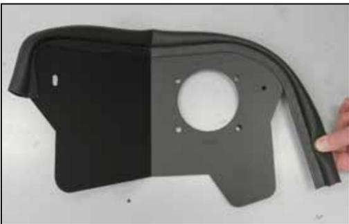
11. Install the supplied edge trim onto the heat shield as shown.
