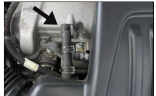
6. Using pliers loosen the clamp which secures the crankcase vent hose to the valve cover vent port and then disconnect the crankcase vent hose as shown.
