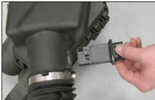
17. Remove the two screws that secure the mass air sensor and then remove the mass air sensor from the stock intake tube as shown.
