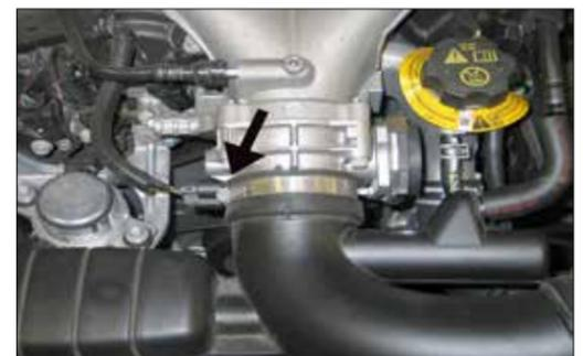
5. Loosen the hose clamp securing the intake tube to the throttle body.
