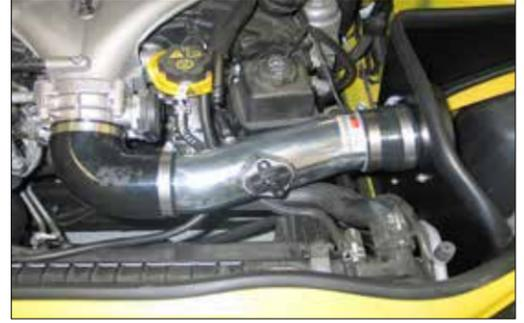
20. Install the K&N intake tube assembly into the silicone hose at the filter adapter and then onto the throttle body, align for proper fit and then secure with the provided hose clamps.
