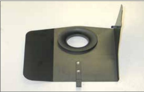
10. Install the filter adapter onto the heat shield and secure with the provided hardware.
