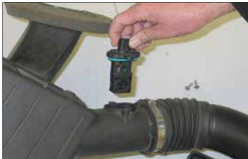
17. Remove the two screws securing the mass air sensor into the factory air box and then remove the mass air sensor from the air box.
