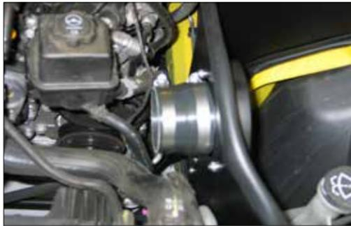
15. Install the provided silicone hose (084091) onto the filter adapter and secure with the provided hose clamp.
