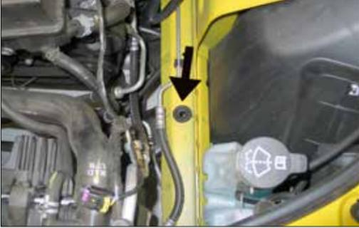
8. Remove the air box mounting grommet shown from the inner fender.
