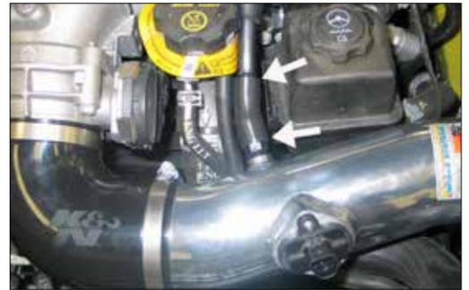
21. Install the provided silicone hose onto the factory crank case vent tube and then connect the open end onto the vent fitting installed into the K&N intake tube.
