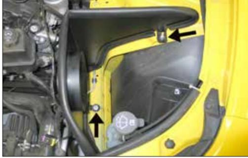
14. Install the heat shield assembly into the vehicle so the inserted nut goes into the air box mounting grommet hole and tab goes onto the air box mounting stud. Secure the heat shield with the provided hardware.
