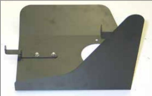
9. Install the provided heat shield mounting bracket (083126) onto the heat shield using the provided hardware.
