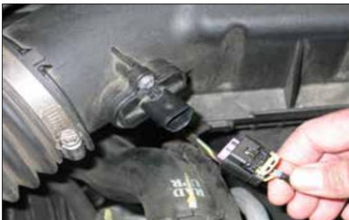
2. Release the locking and then disconnect the mass air sensor electrical connector.
