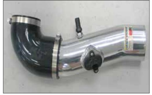
19. Install the provided elbow hose (08629) onto the K&N intake tube as shown and secure with the provided hose clamp.
