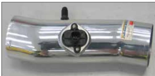
18. Install the mass air sensor into the K&N intake tube and secure with the provided hardware.
