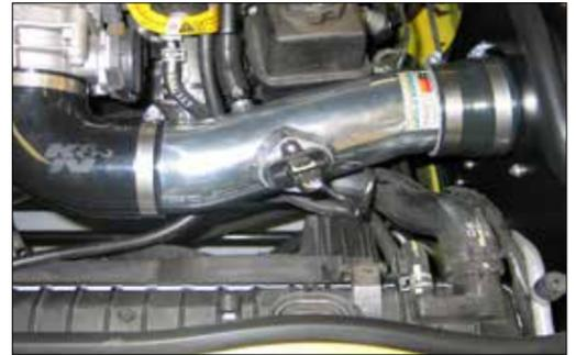
23. Reconnect the mass air sensor electrical connection.
