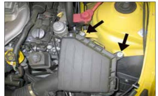
6. Remove the two nuts shown securing the factory air box to the inner fender.
