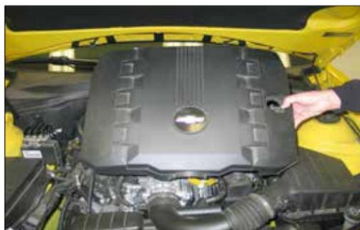
3. Remove the oil fill cap and then remove the engine cover from the engine. Reinstall the oil fill cap.
