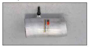
25. Install the provided 1/4npt fitting into the K&N® intake tube as shown.
