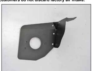
10. Assemble the heat shield half's as shown using the provided hardware.
