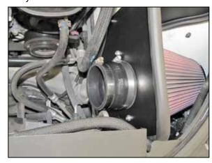
21. Install the provided hose (08051) onto the filter adapter and secure with the provided hose clamp.
