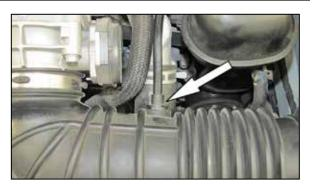
5. Disconnect the crank case vent from the intake tube.
