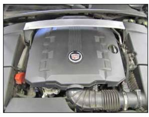
2. Remove the engine oil fill cap and then remove the engine cover. Reinstall the oil fill cap.
