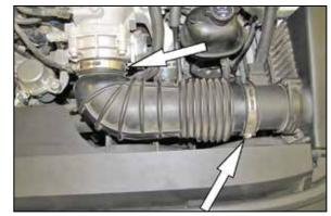
6. Loosen the two hose clamps securing the factory intake hose and then remove the factory intake hose from the vehicle.
