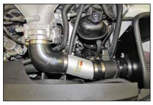
27. Install the tube assembly into the hose at the mass air sensor and align with the throttle body, adjust the tube and elbow hose for best fit and then secure with the provided hose clamps.
