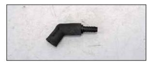
19. Install the provided hose mender into the factory elbow as shown.
