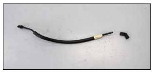
18. Remove the crank case vent tube from the valve cover and then remove the factory elbow from the tube as shown.
