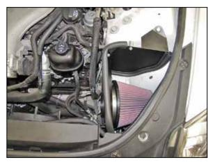
17. Install the heat shield and filter assembly into the engine compartment and secure it the fan shroud with the factory bolt and to the inner fender with the hardware provided.
