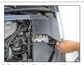
3. Lift up the front of the side cover and then remove the cover from the engine compartment.
