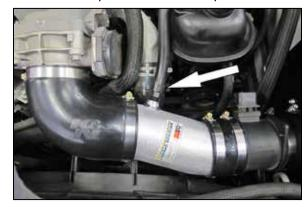
28. Connect the crank case vent hose to the fitting installed into the K&N® intake tube.
