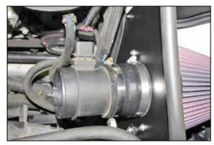
23. Install the mass air sensor housing into the hose at the filter adapter as shown and secure with the provided hose clamp.
