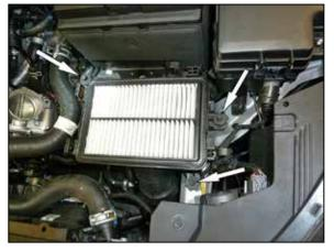
6. Remove the three bolts that secure the lower air filter housing and then remove the lower air filter housing. NOTE: K&N Engineering, Inc., recommends that customers do not discard factory air intake.
