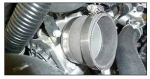
13. Install the provided coupler (08440) onto the throttle body and secure with the provided hose clamp.
