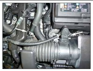
3. Disconnect the mass air sensor electrical connection. Release the spring clamp that secures the PCV hose to the intake hose and then disconnect the PCV hose.
