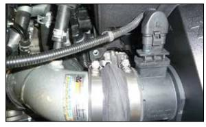
17. Reconnect the mass air sensor electrical connection and connect the factory PCV hose to the fitting installed into the K&N® intake tube.
