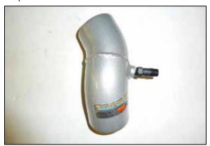
15. Install the provided PCV fitting into the K&N® intake tube as shown.
