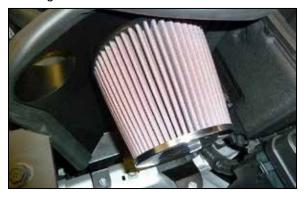
18. Install the air filter onto the mass air sensor housing and secure with the provided hose clamp.
