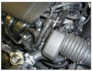
4. Loosen the hose clamp that secures the intake hose to the throttle body.
