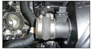
14. Install the provided hump coupler onto the mass air sensor and secure with the provided hose clamp.
