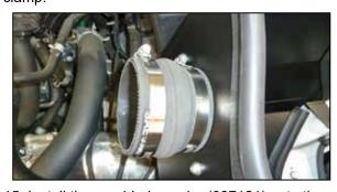
15. Install the provided coupler (087121) onto the filter adapter and secure with the provided hose clamp.
