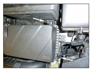
5. Release the two spring clips that secure the upper air filter housing and then remove the upper air filter housing and intake tube from the vehicle.
