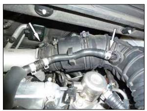
3. Release the spring clamp that secures the PCV vent line and then disconnect PCV line from the intake tube and unhook it from the clip. Loosen the hose clamp that secures the intake to the throttle body.
