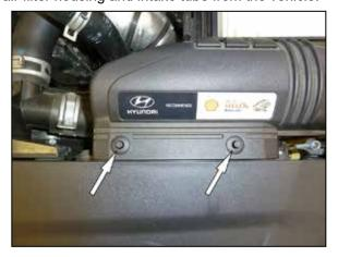
6. Push in the center of the fresh air intake duct retaining pins and then remove the pins from the vehicle.
