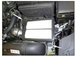
7. Remove the three bolts that secure the lower air filter housing and then remove the housing from the vehicle.
