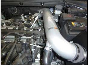
17. Connect the PCV vent and BOV hose to the K&N® intake tube and secure with the factory spring clamps.
