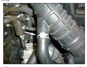
4. Release the spring clamp that secures the BOV hose to the intake tube and then disconnect BOV hose from the intake tube.
