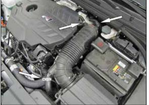
2. Release the spring clamps that secure the breather hoses and BOV hose and then disconnect them from the factory intake tube.
