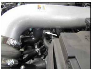
15. Connect the BOV elbow to the K&N<sup>®</sup> intake tube as shown.
