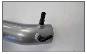
12. Install the provided vent fittings into the K&N<sup>®</sup> intake tube as shown.
