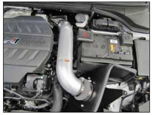
13. Install the K&N<sup>®</sup> intake tube into the coupler at the turbo and then into the coupler at the filter adapter, align the tube for best fit and then secure with the provided hose clamp.
