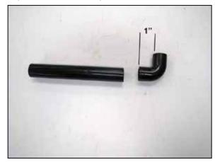
9. Cut the provided BOV hose 1" from the elbow as shown.
