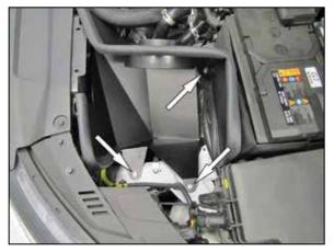
7. Install the heat shield into the vehicle and secure with the provided hardware.
