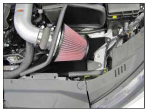
16. Install the K&N<sup>®</sup> air filter and secure with the provided hose clamp.
