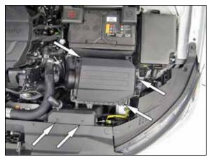
4. Remove the two plastic retaining clips that secure the fresh air intake duct. Remove the three bolts that secure the air filter housing and then remove the assembly from the vehicle. **NOTE: K&N Engineering, Inc., recommends that customers do not discard factory air intake.**  and 34", install the edge trim onto the heat shield as shown.
