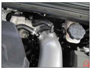
14. Connect the factory vent lines to the fittings installed into the K&N<sup>®</sup> intake tube and secure with the factory spring clamps.
