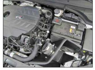
8. Install the provided couplers onto the Turbo inlet (08713) and filter adapter (084079) and secure with the provided hose clamps.
