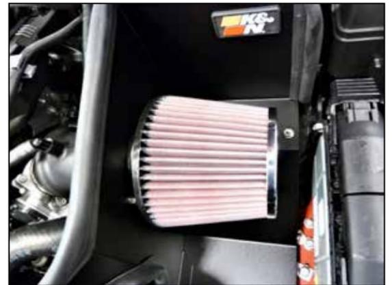
16. Install the K&N air filter onto the mass air sensor and secure with the provided hose clamp.
