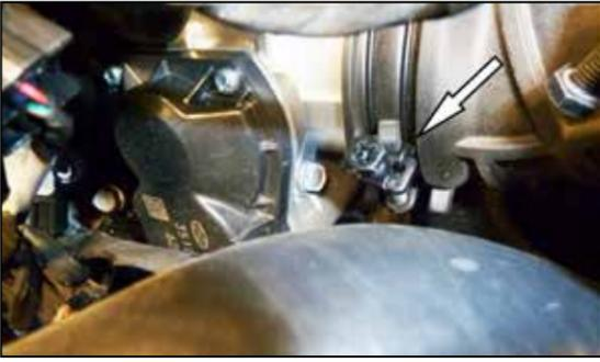
4. Loosen the hose clamp that secures the factory intake tube to the throttle body.
