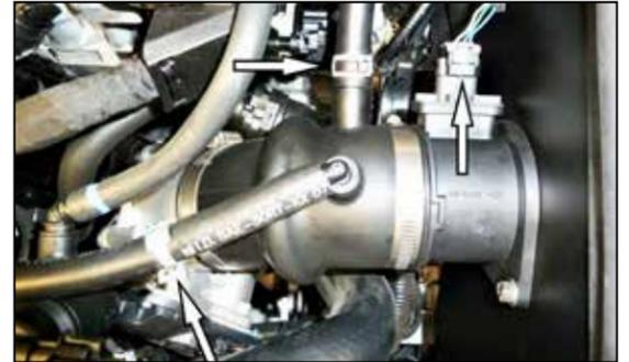
15. Reconnect the vent lines and secure with the factory spring clamps. Reconnect the mass air sensor electrical connection.
