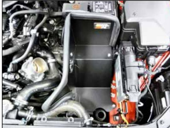
11. Install the heat shield assembly onto the rubber mounted studs and secure with the provided hardware.
