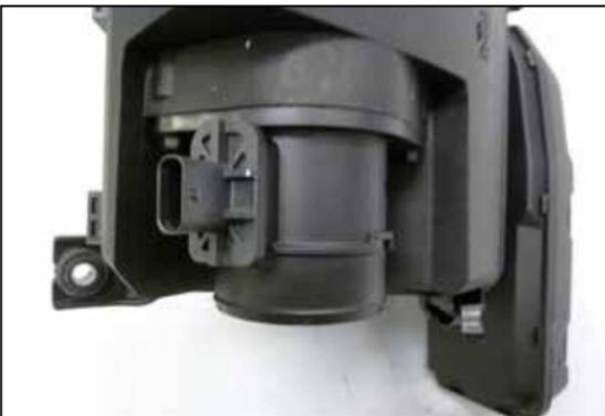
8. Remove the two bolts that secure the mass air sensor to the upper air filter housing and then remove the sensor from the housing.
