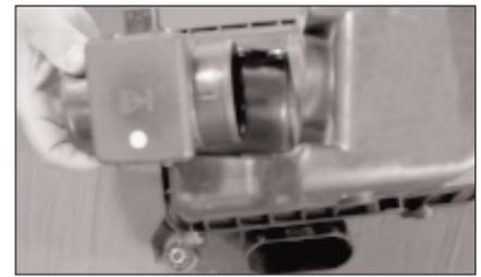
10. Loosen and remove the two bolts that secure the mass air sensor, then remove the mass air sensor as shown.
