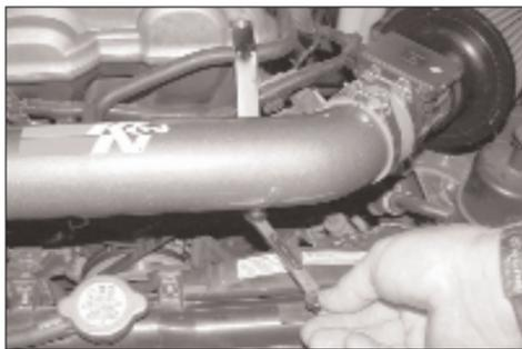
20. Tighten the hex bolt on the K&N® intake tube as shown.
