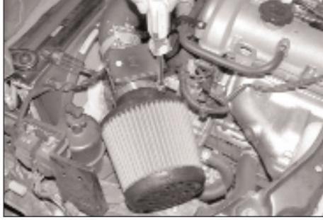
19. Install the K&N® air filter onto the mass air sensor, then, tighten the hose clamp as shown.
