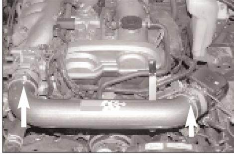
18. Slide the mass air sensor into the silicone hose, then, tighten all hose clamps as shown.
