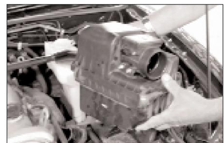
9. Pull upwards to remove the air cleaner assembly as shown. **NOTE: K&N Engineering, Inc., recommends that customers do not discard factory air intake.**
