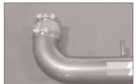
12. Install the silicone step hose and hose clamps onto the K&N intake tube as shown.
