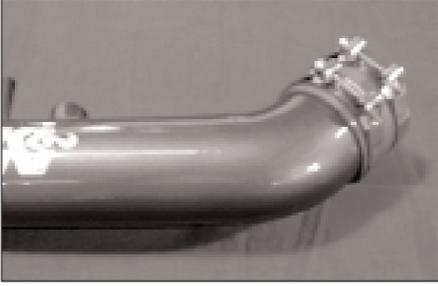
13. Install the silicone straight hose and hose clamps onto the K&N® intake tube as shown.
