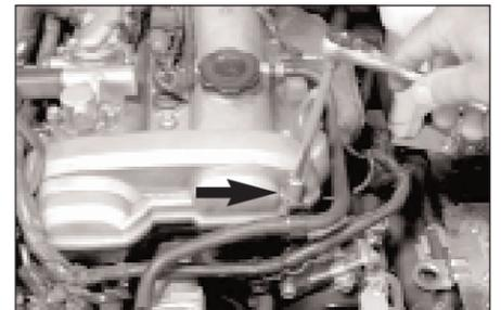
11. Remove the bolt that secures the crankcase vent hose bracket to the cam cover as shown.
