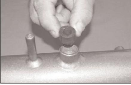
14. Install the silicone sleeve into the air temperature sensor bung on the K&N® intake tube as shown.
