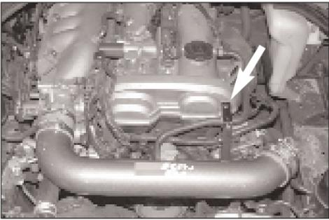
16. Install the K&N® intake tube onto the throttle body, then, line up the bracket with the threaded hole from step 11.
