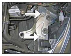
7. Remove the two bolts securing the airbox mounting plate to the inner fender. Remove the mounting plate from the vehicle.
