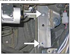
18. Set the two provided ½" spacers onto the inner fender over the airbox mounting bracket bolt holes.
