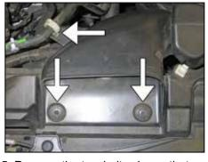
5. Remove the two bolts shown that secure the fresh air duct to the core support, then unhook the coolant hose from the clamp that secures it to the fresh air duct.
