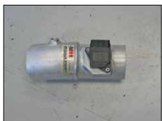
9. Install the mass air sensor into the K&N $^{\circ}$  intake tube and secure with the provided hardware.
