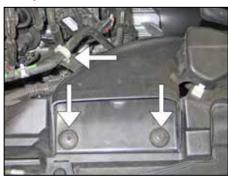
23. Feed the fresh air scoop's outlet into the heat shield while also attaching the inlet back onto the core support. Secure the scoop with the factory bolts that were removed in step #4 and attach the coolant hose with the factory clip.
