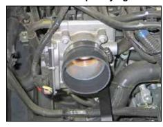
14. Install the provided silicone (084036) hose onto the throttle body and secure with the provided hose clamp.
