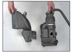
22. Remove the fresh air intake scoop from the factory airbox.
