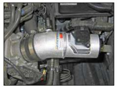
15. Install the K&N® intake tube into the silicone hose on the throttle body and align with the mounting bracket. Secure the tube with the hose clamp and hardware provided.
