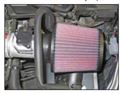
24. Install the K&N® air filter onto the intake tube and secure it in place with the provided hose clamp.
