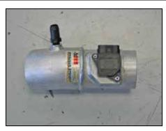
10. Install the 5/8"NPT fitting into the K&N<sup>®</sup> intake tube as shown.
