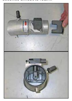
11. Apply a thin coat of the provided super glue to the lip of the air straightener and then install the straightener into the intake tube as shown.
