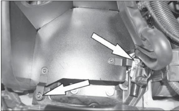
28. Attach the front bracket to the threaded hole on the stock air box mounting point. Attach the fresh air intake door switching valve solenoid and the rear bracket to the other threaded hole with the provided hardware.
