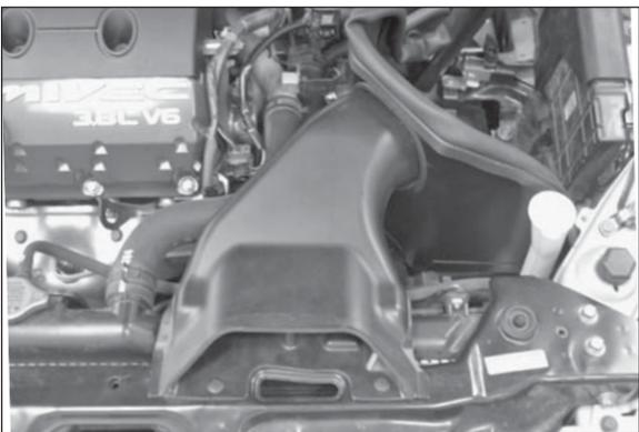
29. Install the factory air inlet duct, and secure with the two screws removed during step # 9. Adjust for fit and clearance, then tighten the heat shield mounting hardware.
