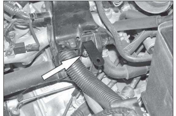
22. Install the "L" Bracket onto the wire harness bracket with the provided hardware.
