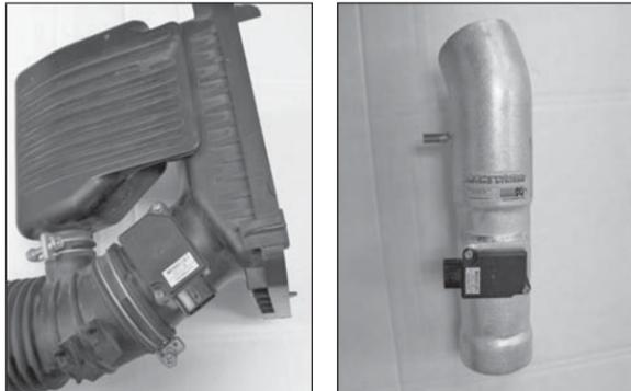
16. Remove the two screws securing the MAF sensor to the factory air box. Install the MAF sensor into the K&N® intake tube with the provided hardware.
