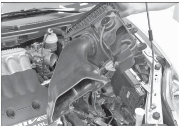
13. Lift the lower air box, pulling up to the left to unclip it.
