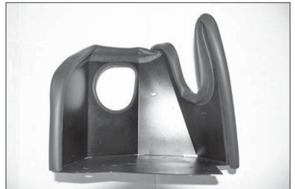
24. Install the small edge trim into the hole, then attach the large edge trim around the heat shield.
