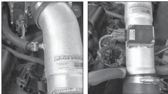
33. Reconnect the crank case vent hose and wire harness to the MAF sensor.
