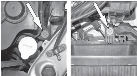
11. Loosen and remove the two bolts that secure the lower air box.
