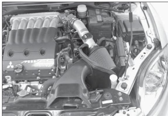
32. Install the K&N® intake tube with the provided hardware as shown. Adjust for best fit and clearance, then tighten all hardware, and hose clamps.
