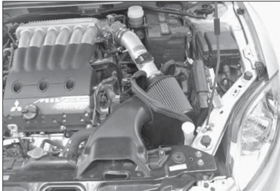
32. Install the K&N® intake tube with the provided hardware as shown. Adjust for best fit and clearance, then tighten all hardware, and hose clamps.
