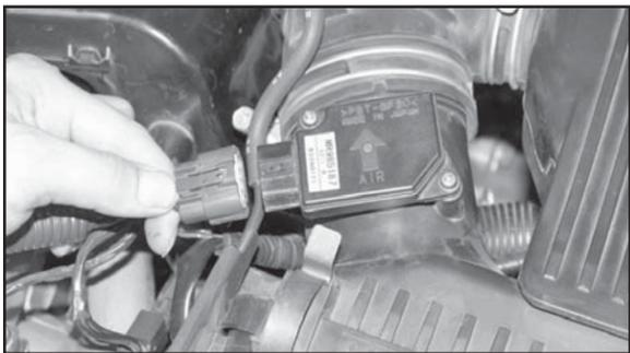
2. Disconnect the MAF sensor harness from the MAF sensor.
