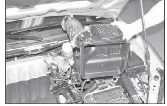
7. Remove the upper air box and intake tube from the vehicle.
