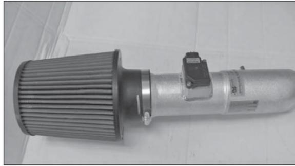
31. Install the K&N® air filter onto the intake tube as shown.
