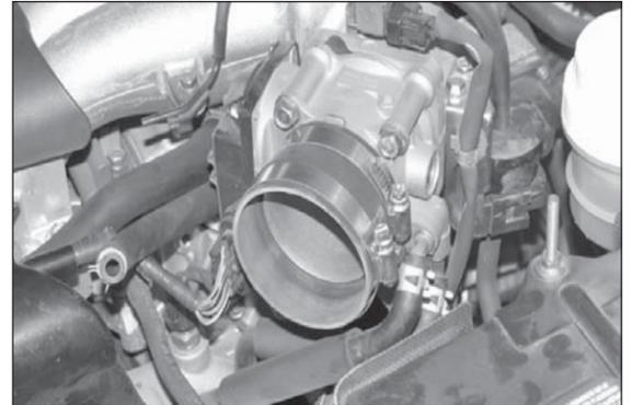
21. Install the provided silicone hose and hose clamps onto the throttle body as shown.
