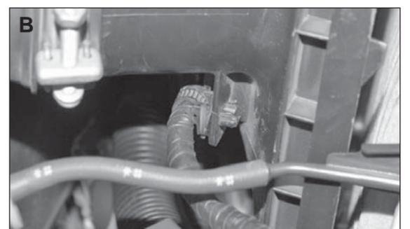
6. Lift the upper air box and turn over (A), then unclip the MAF sensor wire harness (B).
