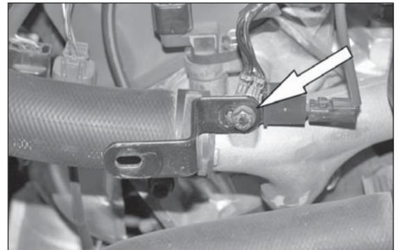
23. Install the "Z" bracket onto the ground with the provided hardware.
