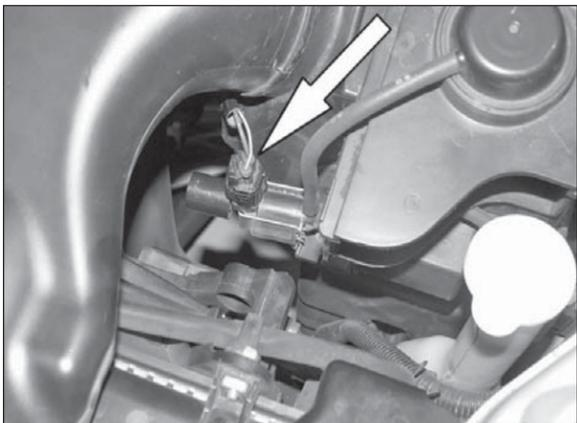
12. Disconnect the fresh air intake door vacuum switch electrical connection.
