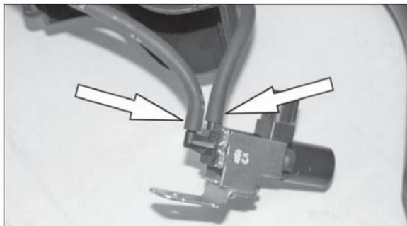
18. Disconnect the vacuum lines from the fresh air door vacuum switching valve.
