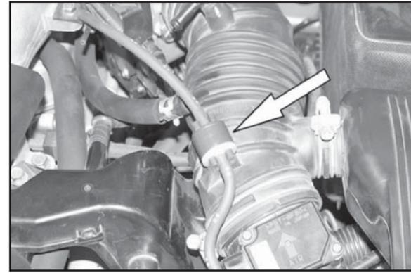
5. Unclip the Vacuum Switching Valve hose from the stock intake tube.
