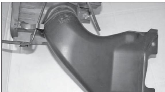
19. Unclip and remove the air inlet duct from the lower air box.
