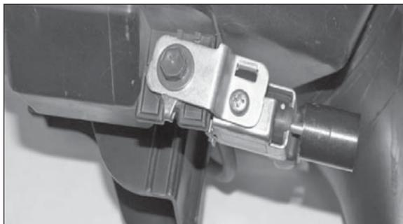
17. Loosen and remove the bolt that secures the fresh air intake door switching valve solenoid to the lower air box.
