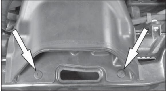
9. Loosen and remove the 2 screws that hold the air inlet duct in place.
