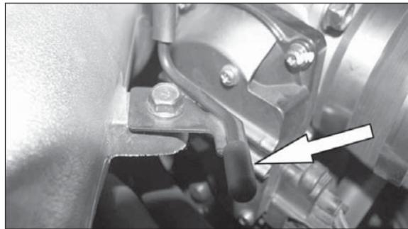
3a. Plug the fresh air intake door vacuum port with the provided rubber cap.
