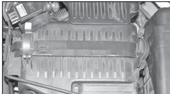
4. Unclip the two clips that hold the air box together.
