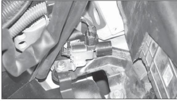
30. Reconnect the fresh air intake door vacuum switching valve solenoid electrical connection.
