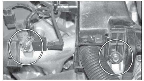
20. Loosen and remove the two specified bolts. (Ground and wire harness)
