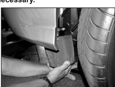
32. From underneath the vehicle install the K&N® air filter onto the cold air tube and secure with the provided hose clamp as shown.
