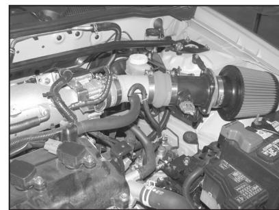
40. This K&N® high flow intake system has been designed to be used in two different configurations. In the case of inclement weather, the cold air tube can be removed and the air filter can be clamped onto the intake tube located in the engine compartment to avoid the possibility of ingesting water into the engine.
