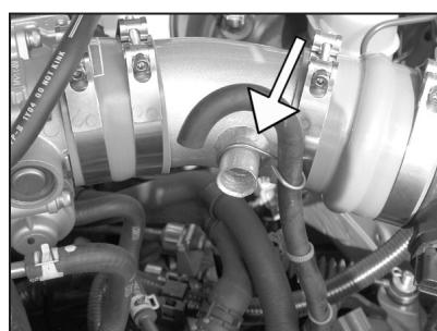
34. Slide the wire hanger onto the vent on the throttle body tube as shown.
