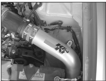
28. Line up the silicone hose on the cold air tube with the mass air sensor adapter, then slide the silicone hose onto the adapter and tighten with the provided hose clamp as shown.
