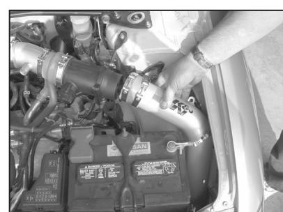
27. Slide the cold air tube into the hole on the inner fender as shown.
