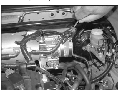
15. Install the silicone hose and hose clamps onto the throttle body, then, tighten the hose clamp on the throttle body as shown.
