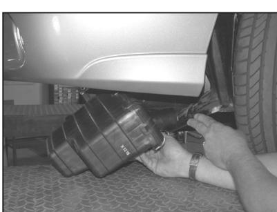
14. From underneath the vehicle loosen and remove the two bolts that secure the air intake resonator, then, remove the resonator as shown.
