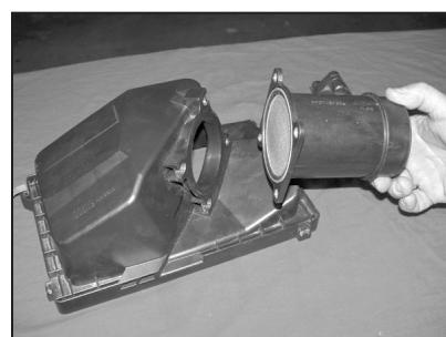
18. Loosen and remove the four bolts that secure the mass air sensor to the air cleaner, then remove the mass air sensor as shown.
