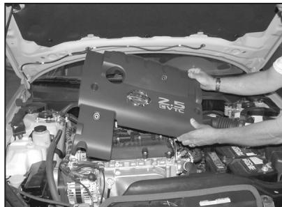
2. Remove the four bolts that secure the engine cover, then remove the engine cover as shown.
