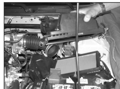
8. Unclip the upper air cleaner assembly, then remove the assembly as shown.
