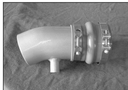
16. Install the stepped hump hose and hose clamps onto the throttle body tube and tighten as shown.
