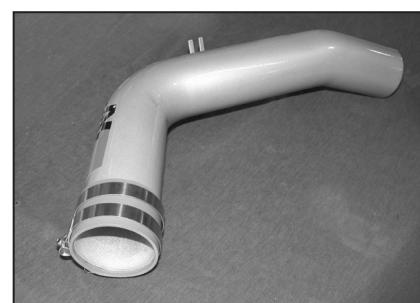
25. Install the silicone hose and hose clamps onto the K&N cold air tube as shown.
