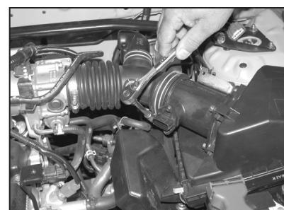
7. Loosen the hose clamp at the mass air sensor as shown.
