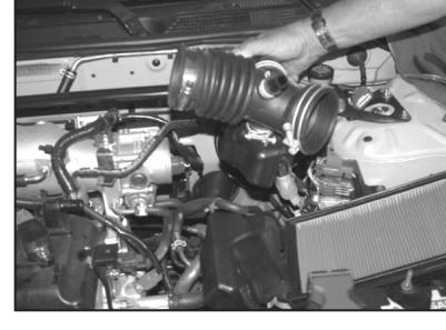
9. Loosen the hose clamp at the throttle body, then remove the stock intake tube as shown.
