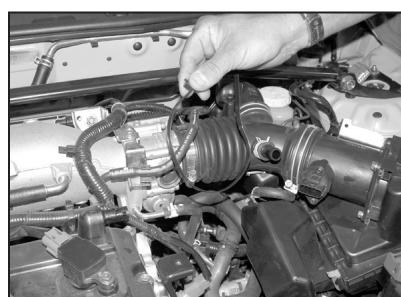
6. Remove the tie-wrap that secures the electrical connection to the rubber intake tube as shown.
