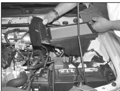
11. Loosen and remove the bolt that secures the lower air cleaner assembly, then, pull upwards to remove the assembly as shown.
