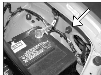
23. Install the remaining rubber mounted stud into the threaded hole on the inner fender as shown.
