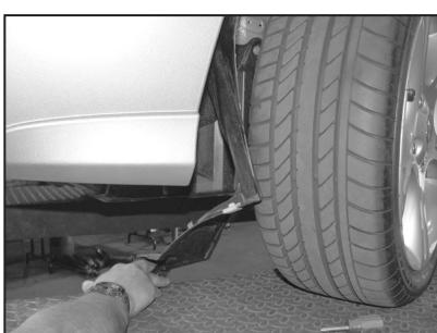
13. Remove the one screw and four push clips on the inner fender valance, then pull the valance down as shown.
