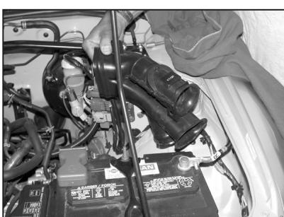
12. Pull upwards to release the air inlet duct, then slide the air inlet duct out as shown.
