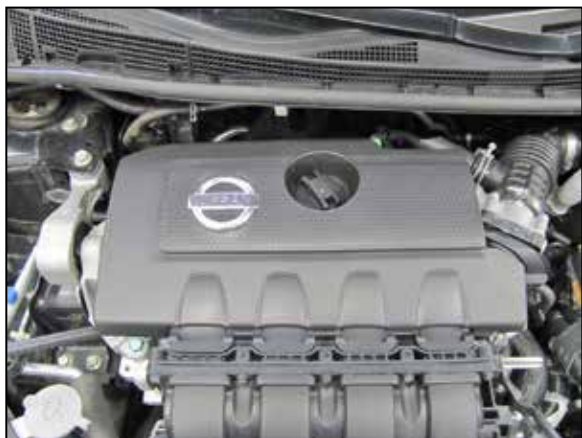
2. Lift up and remove the engine cover.
