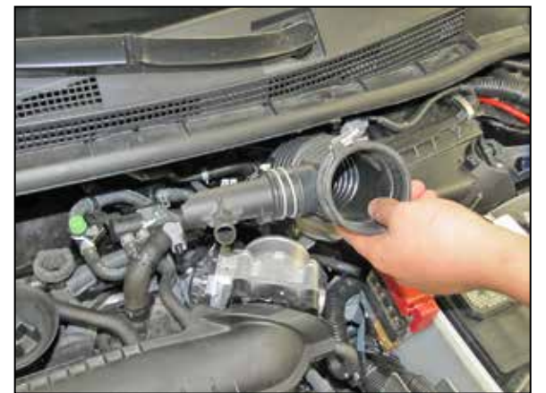
5. Remove the intake hose from the vehicle.
