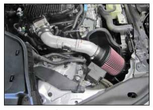
26. Install the K&N® air filter and secure with the provided hose clamp. Adjust the intake tube, heat shield and filter for pest fit and then secure all of the mounting points.
