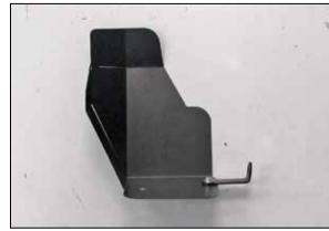
15. Install the mounting bracket (070109) onto the passenger side heat shield (073171) as shown and secure with the provided hardware.
