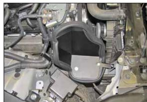
19. Install the provided straight vent fitting into the passenger side K&N® intake tube (27620) as shown.
