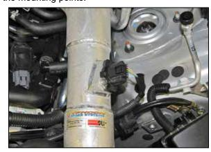
41. Reconnect the mass air sensor electrical connection.
