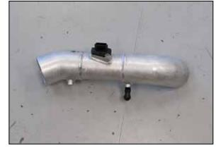
35. Install the mass air sensor into the K&N® intake tube and secure with the provided hardware.
