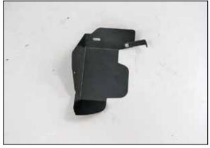
29. Install the heat shield mounting bracket (070109) onto the driver's side heat shield (073172) and secure with the provided hardware.
