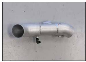
33. Install the provided  $90^{\circ}$  vent fitting into the passenger side  $K\&N^{\circ}$  intake tube (27620) as shown. NOTE: NPT fitting has tapered threads and only designed to be installed until hand tight, then tighten one rotation or when the fitting becomes difficult to return.
