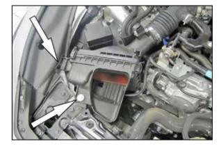
5. Remove the two bolts that secure passenger side air box and loosen the hose clamp to the intake tube.
