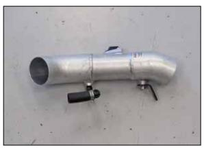
38. Install the tube mounting bracket (070049) onto the K&N® intake tube and secure with the provided hardware.
