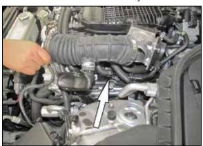
13. Pull the intake hose up to gain access to the crank case vent to valve cover connection. Release the clamp securing the crank case vent and then remove the driver's intake hose assembly.
