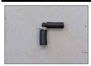
36. Install the 5/8" and 1/2" crank case vent hose's onto the ½" 90° fitting.
