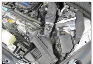
9. Disconnect the driver side mass air sensor electrical connection and unhook the wiring harness from the air box.
