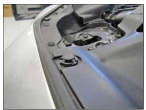
3. Release the eight clips securing the core support decorative cover and then remove the cover from the vehicle.
