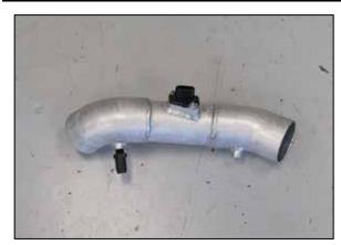
21. Install the mass air sensor into the K&N® intake tube and secure with the provided hardware.
