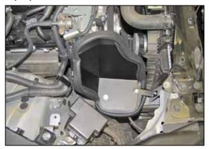
18. Install the heat shield into position as shown on the passenger side frame rail and then secure to the core support with the provided hardware. NOTE: The mounting stud will insert into the factory air box mounting grommet.
