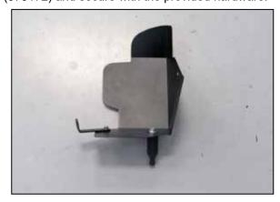
30. Install the provided mounting stud onto the driver's side heat shield and secure with the provided hardware.
