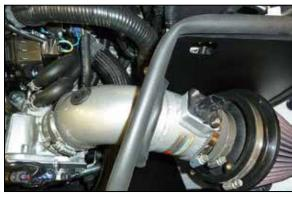
17. Install the intake tube through the heat shield and into the coupler at the throttle body, adjust the tube for best fit and then secure with the provided hose clamp.
