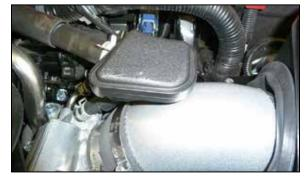
18. Install the PVC chamber into the grommet in the K&N® intake tube.
