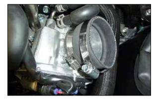
13. Install the provided coupler (08186) onto the throttle body and secure with the provided hose
