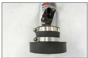
15. Remove the mass air sensor from the factory housing and then install it into the K&N® intake tube and secure with the provided hardware. Install the coupler (084036) onto the K&N® intake tube and then install the filter adapter into the coupler and secure them with the provided hose clamp.
