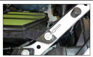
7. Remove the bolt that secures the lower air filter housing and then remove the housing from the vehicle.
