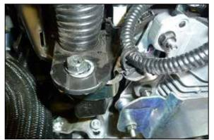
11. Remove the bolt that secures the wiring harness shown.
