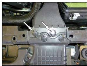
6. Remove the two plastic clips that retain the fresh air intake duct and then remove the duct from the vehicle.
