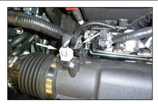
3. Disconnect the mass air sensor electrical connection and then unhook the harness from the air filter housing and engine.
