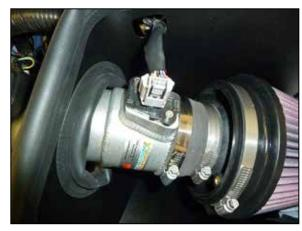
19. Reconnect the mass air sensor electrical connection.
