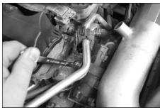
22. Align the bracket the A-tube with the rubber vibration stud and secure it using an M6 Nylock nut and flat metal washer supplied. Do not fully tighten yet!
