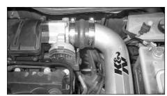
21. Feed the A-tube into the silicone hump hose and secure it with a #40 hose clamp supplied. Do not fully tighten yet! .
