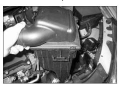
5. Remove the complete air box assembly from the vehicle by pulling it firmly upwards.
