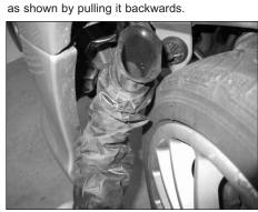
11. Carefully remove the cold air intake snorkel from the inner wing as shown.
