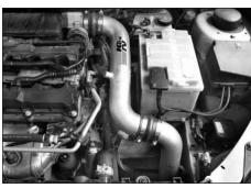
26. Align the A- and B-tube for best fit and clearance; now firmly tighten all hose clamps and hardware.
