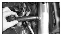
30. Fit the supplied silicone breather hose between the breather assembly and the breather pipe of the A-tube as shown.
