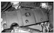
2. Unbolt and remove the engine cover from the vehicle.
