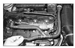
3. Remove the breather assembly from the vehicle as shown; press the yellow tabs to release.
