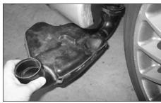
10. Remove the resonator box from the vehicle
