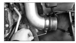
23. Secure the silicone hump hose onto the Atube using a #40 hose clamp supplied.
