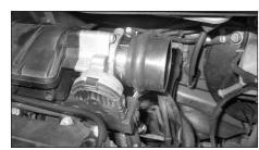
17. Fit the silicone hump hose onto the throttle body as shown, and secure using a #40 hose clamp supplied.
