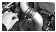
24. Feed the B-tube into the silicone hump hose and secure using a #40 hose clamp supplied. Do not fully tighten yet!
