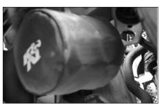
28. Fit the filter/drycharger assembly onto the B-tube using the #40 hose clamp supplied.
