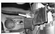
12. Remove the bolt securing the air box mounting bracket to the vehicle.
