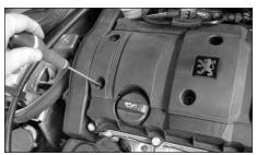
31. Re-install the engine cover to the engine, using the original hardware.
