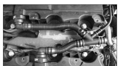
16. Re-install the breather assembly onto engine.
