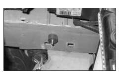
14. Screw the rubber vibration stud provided into the threaded air box mounting point from step 12 as shown.
