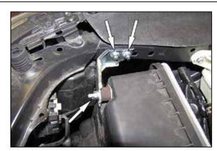
5. Remove the three nuts that secure the air filter
