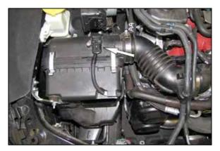
3. Disconnect the mass air sensor electrical
