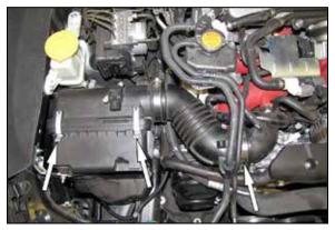
4. Loosen the hose clamp that secures the intake hose to the turbo inlet. Release the air filter housing clam shell clips and then remove the air filter clean side housing, intake hose and factory air filter from the vehicle.
