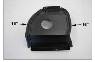
8. Install the edge trim onto the heat shield as shown.
