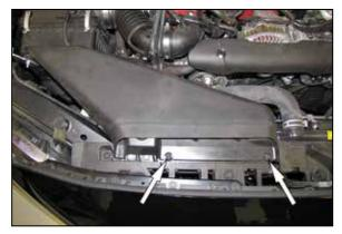
2. Remove the two plastic retaining clips that secure the fresh air duct and then remove the fresh air duct from the vehicle.
