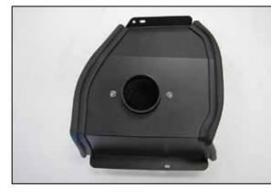
10. Install the filter assembly into the heat shield assembly and secure with the provided hardware.
