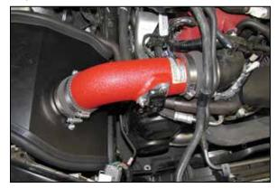
14. Install the K&N<sup>®</sup> intake tube into the coupler at the turbo inlet tube and align with the filter adapter, slide the coupler onto the filter adapter, adjust the tube for best fit and secure with the hose clamps. Secure the heat shield with the provided hardware.
