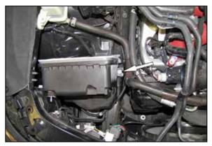
6. Remove the bolt that secures the dirty side air filter housing to the frame rail and then remove the air filter housing from the vehicle.
