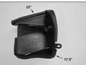
15. Install the 17.5" section to the rear edge of the heat shield and the 22"section to the front edge.
