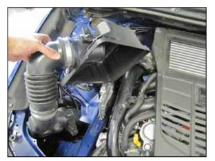
7. Separate the intake tube from the turbo inlet tube and remove the complete assembly from the vehicle.
