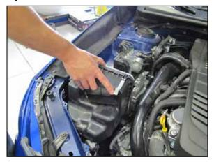
4. Release the two retaining clips and then remove the front half of the air filter housing and the factory air filter. 5. Disconnect the mass air sensor electrical connection.
