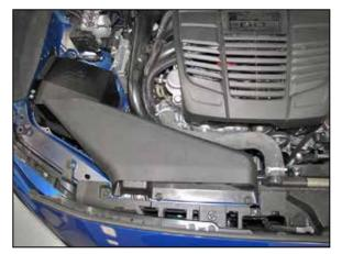
17. Reinstall the fresh air intake scoop so the outlet engages with the heat shield then secure with the factory retaining clips.
