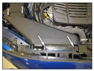
2. Remove the two retaining clips that secure the fresh air intake scoop and then remove the fresh air intake scoop from the vehicle.
