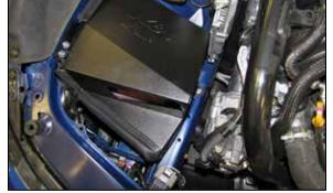
16. Install the heat shield onto the rubber mounted stud and the studs on the inner fender, secure with the factory nuts and hardware.
