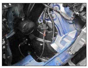
12. Connect the mass air sensor electrical connection using the provided extension harness.
