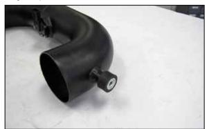
9. Install the provided rubber mounted stud onto the  $K\&N^{\otimes}$  intake as shown.
