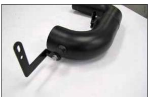
10. Install the provided tube mounting bracket (064359) onto the intake tube and secure with the provided hardware as shown.
