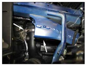
6. Loosen the hose clamp that secures the factory intake tube to the factory turbo inlet tube and remove the nut mounting the tube to the frame. NOTE: the nut is under the frame member. This nut will be reused in a later step.
