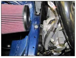
13. Install the K&N<sup>®</sup> air filter onto the intake tube and secure with the provided hose clamp. Install the provided rubber mounted stud onto the frame in the factory air filter housing mounting location as shown.
