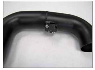
8. Remove the mass air sensor from the Factory intake tube and install it in to the K&N<sup>®</sup> intake tube using the provided hardware.
