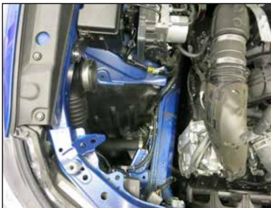
7. Remove the remaining air filter housing half from the engine compartment.
