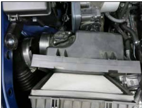
6. Loosen the hose clamp that secures the intake tube to the air filter housing and disconnect the hose. Release the two retaining clips and then remove the housing half and factory air filter.
