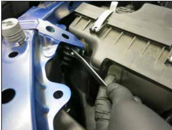
5. Remove the nut that secures the vibration damper to the core support. This nut will be reused in a later step.
