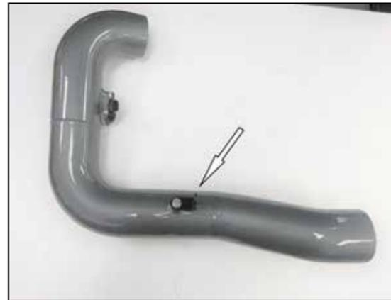
14. Install the provided mounting bracket onto the intake tube as shown using the provided hardware.
