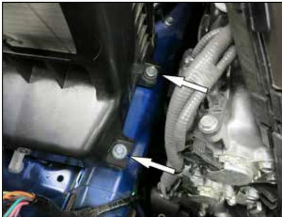
4. Loosen and remove the two bolts that secure the factory air filter housing to the inner fender.
