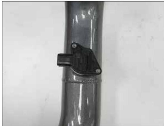
13. Remove the mass air sensor from the factory housing and install it into the K&N intake tube using the provided hardware.
