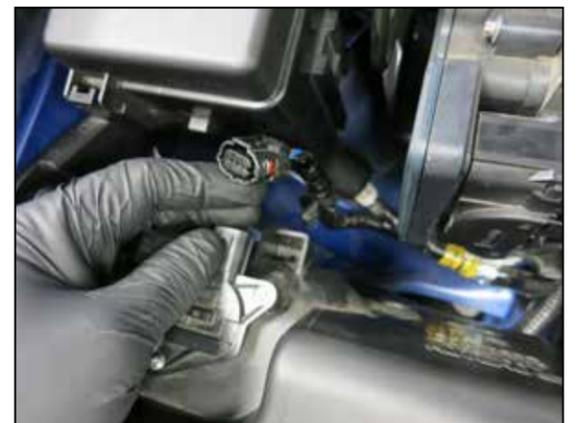
3. Disconnect the mass air sensor electrical connection and unhook the wiring harness from the air filter assembly.
