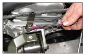
9. Remove the bolt that secures the wire harness bracket to the engine mount bracket as shown.
