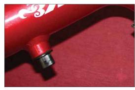
11. Install the air temperature sensor into the silicone hose on the intake tube as shown.
