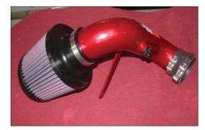
13. Install the air fitler onto the intake tube as shown.
