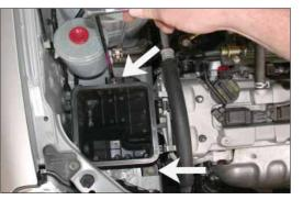
6. Remove the two bolts that secure the lower air cleaner assembly.
