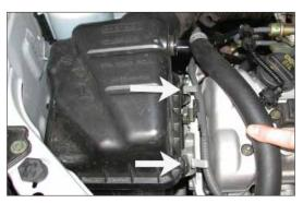
4. Unclip the upper air cleaner assembly as shown.
