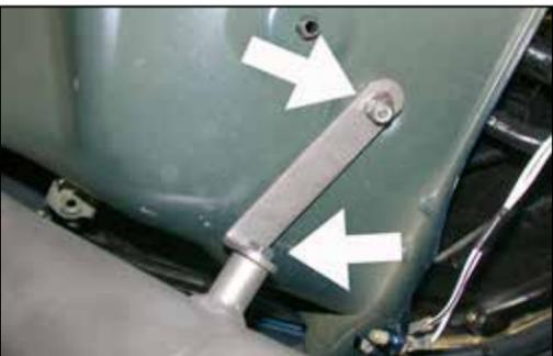
29. Install the provided bracket onto the tube with the provided hardware, then, secure the bracket to the hex bolt from step 28 as shown above.
