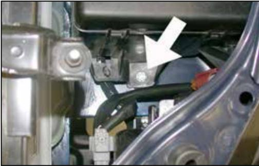
28. Install the provided hex bolt into the fuse box mount from the previous step as shown.
