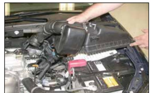
9. Depress the spring clamp on the throttle body, then, remove the complete upper air cleaner assembly as shown.
