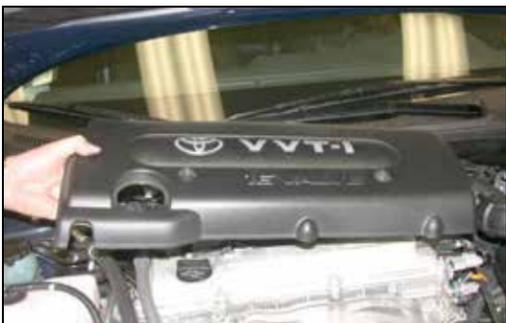
2. Remove the engine cover, which is secured by two acorn nuts as shown.
