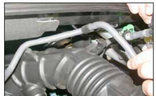
7. Unclip the vent hose from the stock intake tube as shown.
