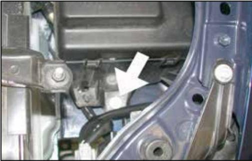
27. Remove the lower fuse box hex bolt as shown above.
