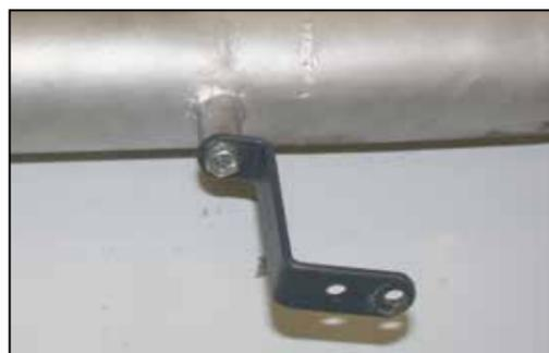
19. Install the provided bracket onto the K&N® intake tube and secure with the provided hardware, but do not tighten completely at this time.
