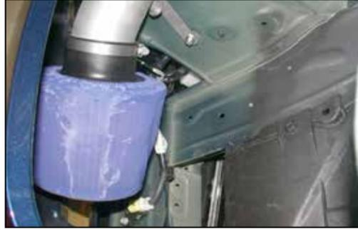
31. Slide the K&N® air filter onto the K&N® cold air tube and secure with the provided hose clamp as shown.
