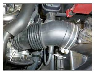
3. Release the spring clamp that secures the intake tube to the throttle body and then disconnect the hose from the throttle body. Disconnect the vacuum line from the intake tube.
