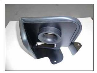
7. Install the provided edge trim onto the heat shield as shown. NOTE: Some trimming of the edge trim will be necessary.
