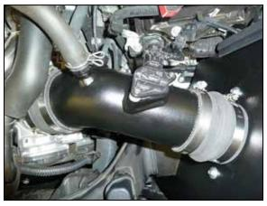
13. Install the intake tube into the previously installed couplers, adjust the tube for best fit and secure with the provided hose clamps. Reconnect the mass air sensor electrical connection. Connect the vacuum line and crank case vent line to the K&N® intake tube.
