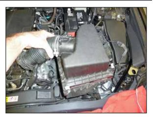
5. Lift the air filter housing up to dislodge it from the mounting grommets and remove the complete assembly from the vehicle. **NOTE: K&N Engineering, Inc., recommends that customers do not discard factory air intake.**
