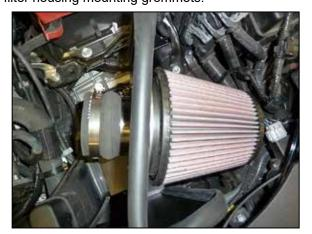
10. Install the provided hump coupler onto the filter adapter and secure with the provided hose clamp. Install the K&N® air filter onto the filter adapter and secure with the provided hose clamp.
