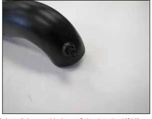
6. Install the provided vent fitting into the  $K\&N^{\otimes}$  intake tube as shown.
