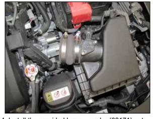
4. Install the provided hump coupler (08171) onto the filter housing and secure with the provided hose clamp.
