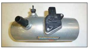
8. Remove the mass air sensor from the factory housing and install it into the K&N® intake tube and secure with the provided hardware.
