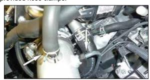
18. Connect the crank case vent line and vacuum line to the vent fittings installed into the K&N® intake tube.
