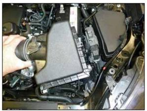
6. Pull upwards on the air box assembly and remove it from the vehicle.
