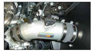
17. Install the K&N<sup>®</sup> intake tube assembly into the couplers and adjust for best fit and secure with the provided hose clamps.
