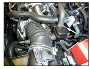
4. Disconnect the Crank case vent line and small vent line shown.
